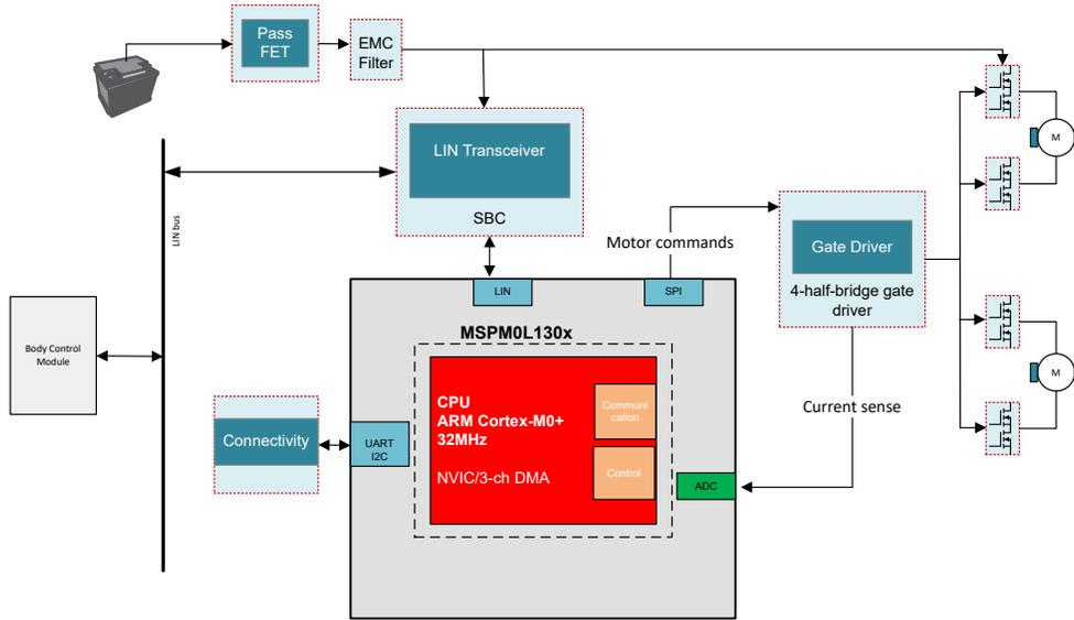
**Figure 4. MSPM0 Dual-Window Drive Module System Block Diagram**
