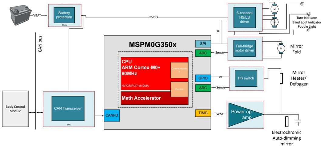
**Figure 5. Side Mirror Module System Block Diagram**
