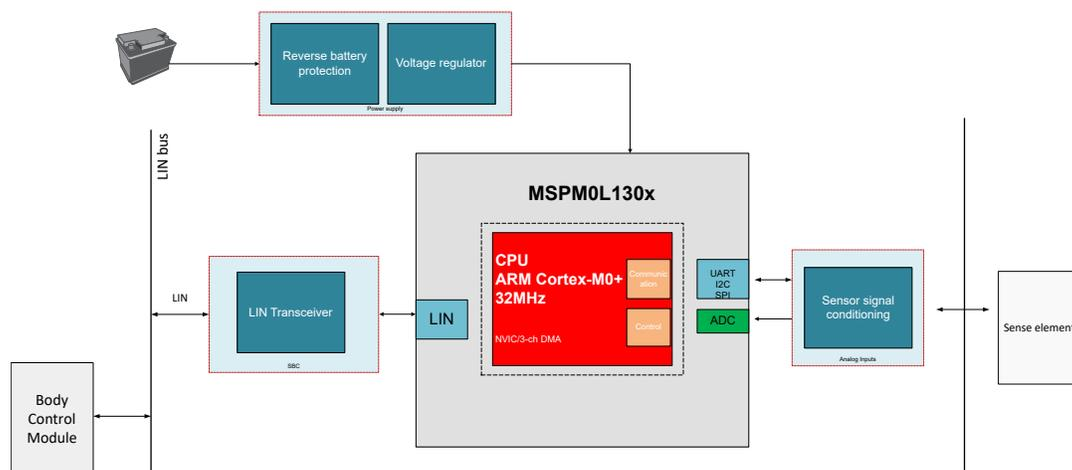
Figure 6. MSPM0 Kick to-open-Trunk Module System Block Diagram
