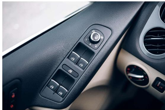
Figure 2. Windows and Mirror Control Switches
