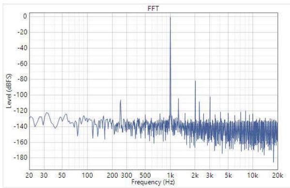
Figure 2-21. Output with IN1P Mux Input Configured
