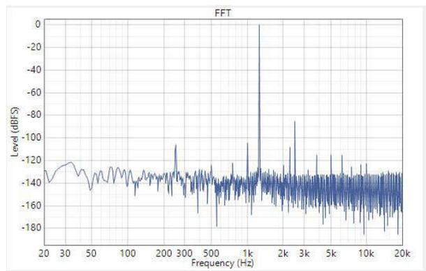
Figure 2-22. Output with IN1M Mux Input Configured
