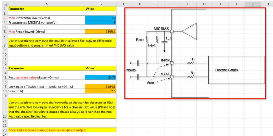
**Figure 2-1. AC-Coupled External Resistor Calculator**
