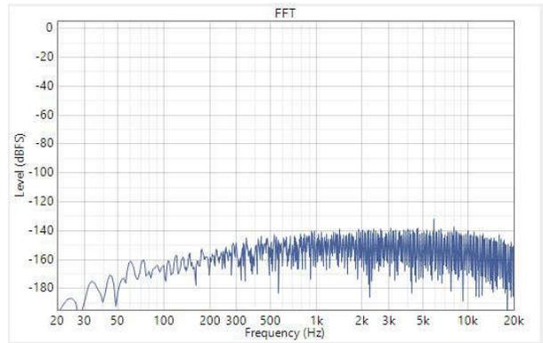
**Figure 2-13. SNR with Input AC Signal shorted to GND**
