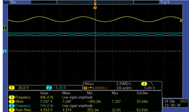
Figure 3-2. IN1P and IN1M Input Signal
