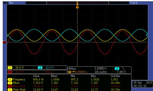
**Figure 2-3. Differential AC-Coupled Input Swing at -1dBrG (0dBrG = 10Vrms)**
