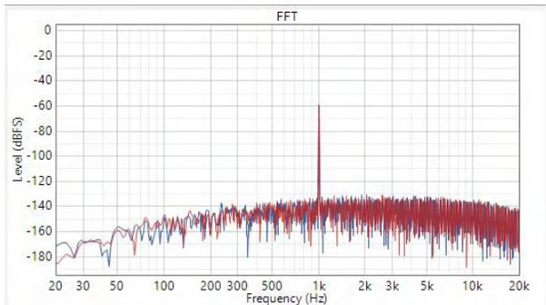
**Figure 2-16. Single Ended DC Coupling Dynamic Range with -60dB<sub>RG</sub> Input**
