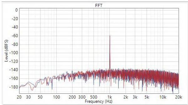
**Figure 2-4. Differential AC-Coupled Dynamic Range at -60dB<sub>r</sub>G Input**
