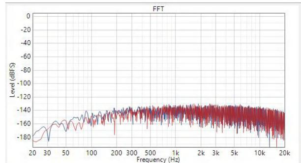
**Figure 2-9. SNR with Input AC Signal shorted to GND**
