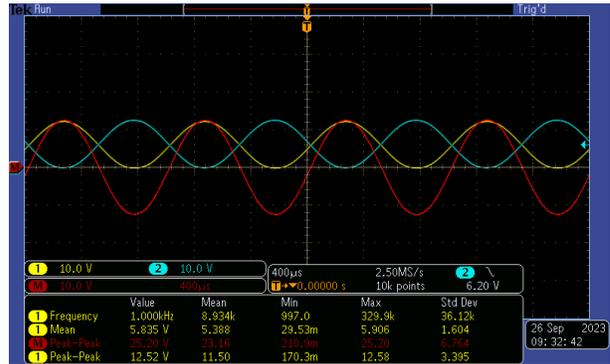
**Figure 2-11. Differential DC-Coupled Input Swing at -1dBrG (0dBrG = 10Vrms)**
