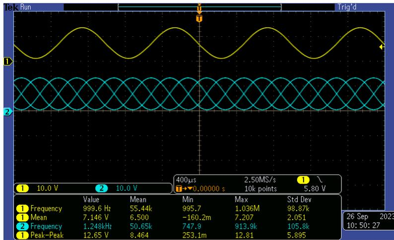
Figure 2-20. IN1P and IN1M Mux Input at -1dBrG (0 dBrG = 5Vrms)
