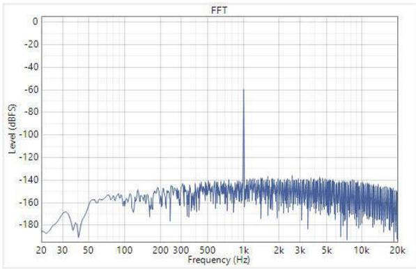
**Figure 2-12. Differential DC-Coupled Dynamic Range at -60dBrG Input**
