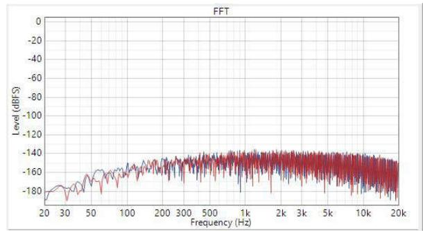
**Figure 2-5. SNR with Input AC Signal shorted to GND**
