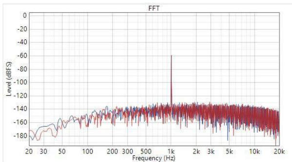
**Figure 2-8. Single Ended AC-Coupled Dynamic Range at -60dBrG Input**
