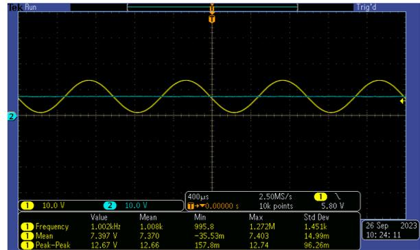
**Figure 2-7. Single Ended AC-Coupled Input Swing at -1dBrG (0dBrG = 5 Vrms)**
