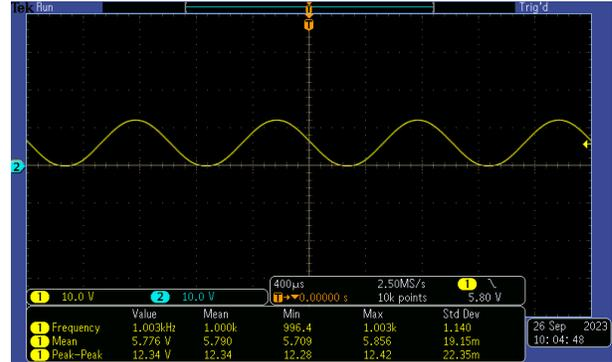
**Figure 2-15. Single Ended DC-Coupled Input Swing at -1dB<sub>RG</sub> (0dB<sub>RG</sub> = 5V<sub>rms</sub>)**
