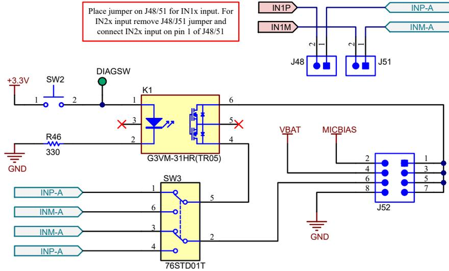
Figure 2-14. TA5x1x-Q1 EVM Diagnostic Circuitry
