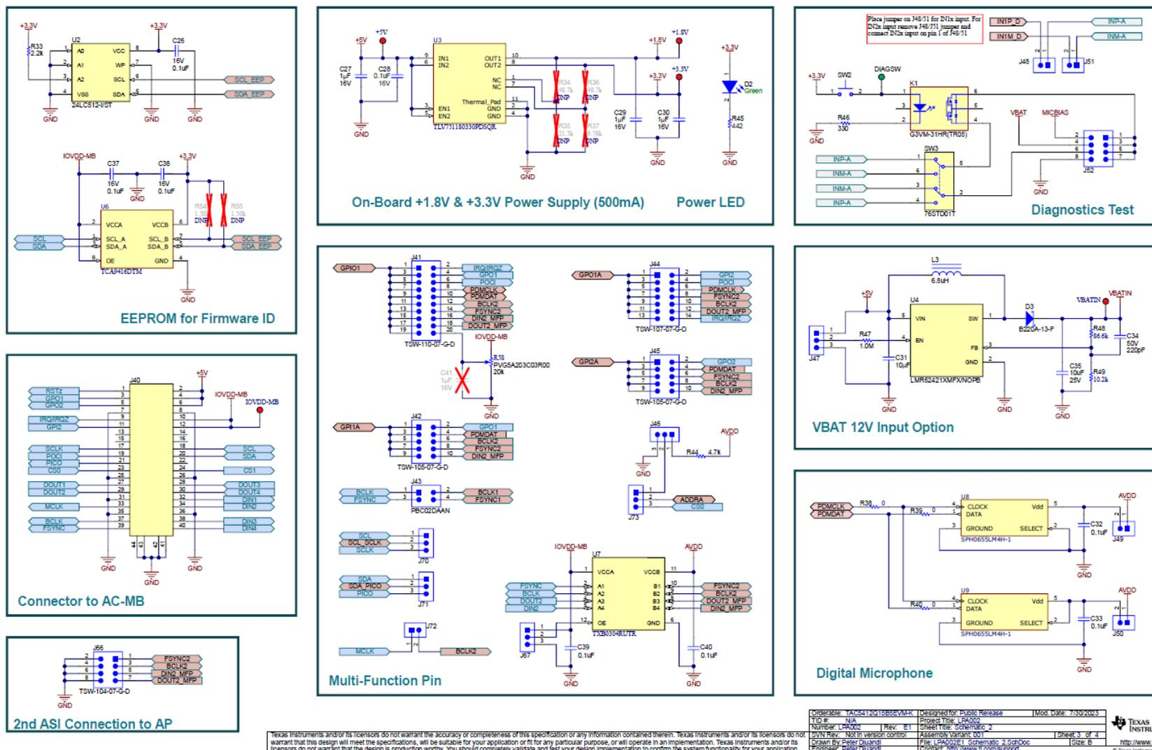
Figure 4-2. TAC5412-Q1 EVM Connectors and Supporting Circuitry Schematic
