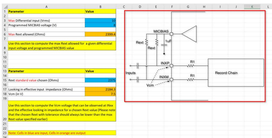
Figure 2-11. AC-Coupled External Resistor Calculator
