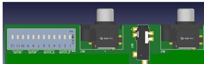
**Figure 2-13. TAC5x12-Q1 Analog Output Connections**
