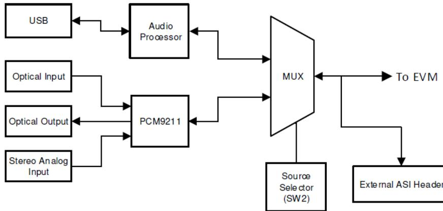
**Figure 2-3. AC-MB Audio Interface Block Diagram**
