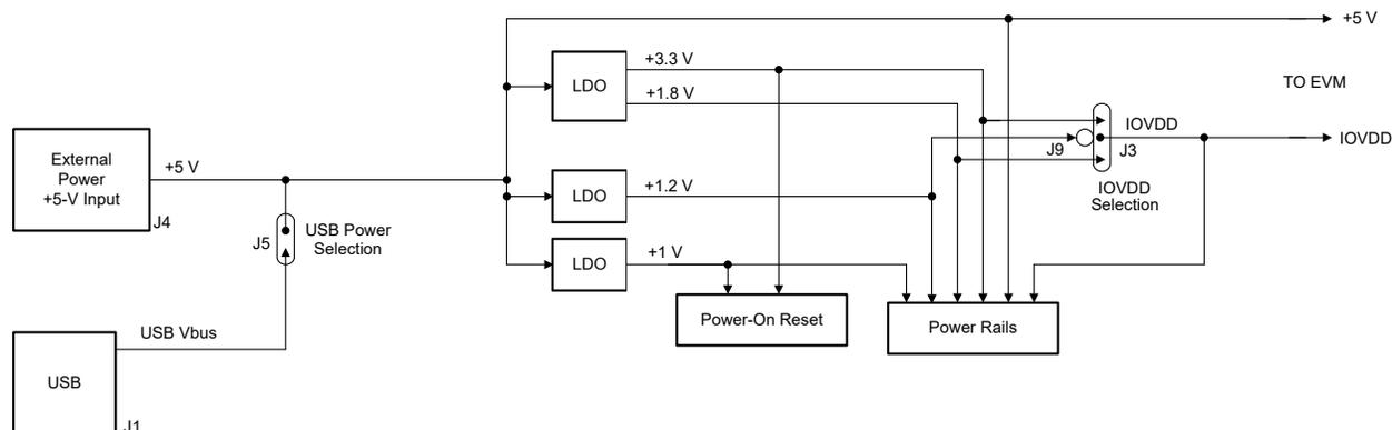
**Figure 2-8. Power-Supply Distribution of the AC-MB**
