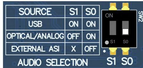
**Figure 2-6. AC-MB External Audio Interface Setting**
