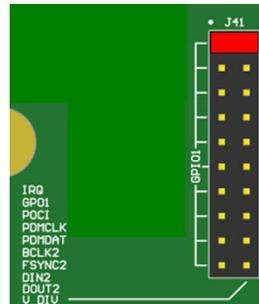
Figure 2-20. GPIO1 Configuration
