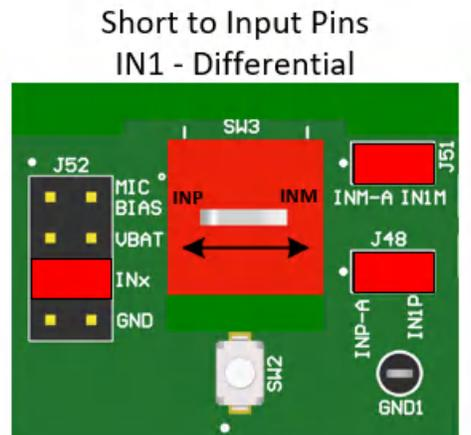
Figure 2-18. Short to Input Diagnostic Test Setup
