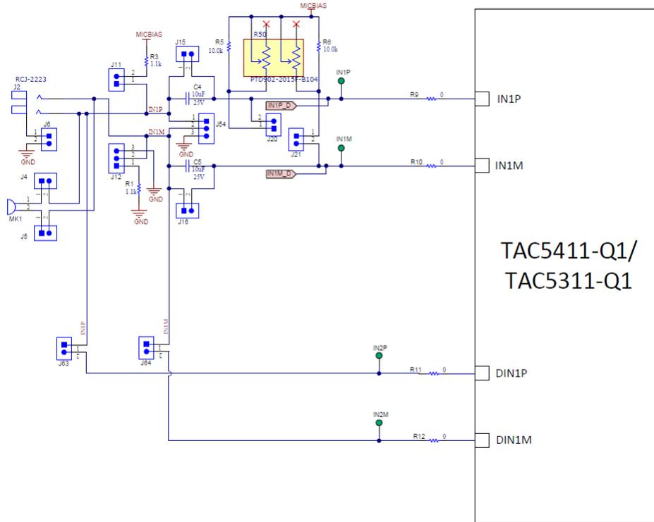
Figure 2-10. TAC5x11-Q1 EVM Input Architecture for Channel 1 and DIN1P/M
