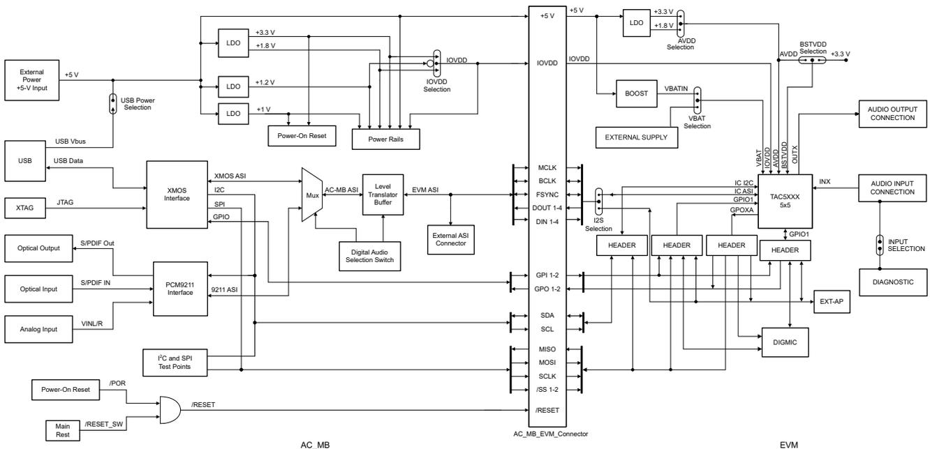
Figure 2-2. TA5x1XQ1 EVM Block Diagram
