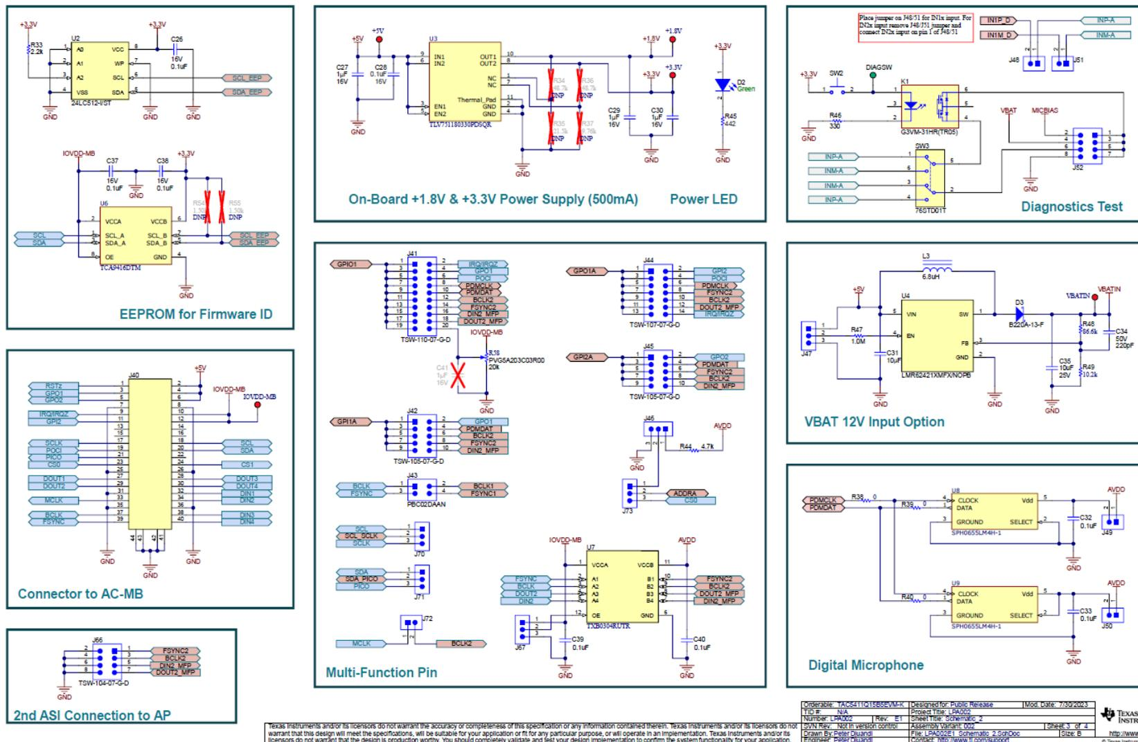
Figure 4-4. TAC5411-Q1 EVM Connectors and Supporting Circuitry Schematic
