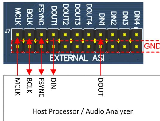
**Figure 2-7. AC-MB Connection with External Audio Serial Interface**
