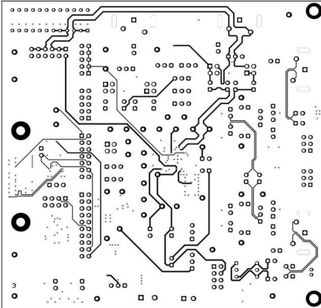
Figure 4-11. TAC541x-Q1 EVM Signal Layer 1
