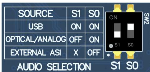
Figure 2-5. AC-MB Optical or Auxiliary Analog Audio Input Setting
