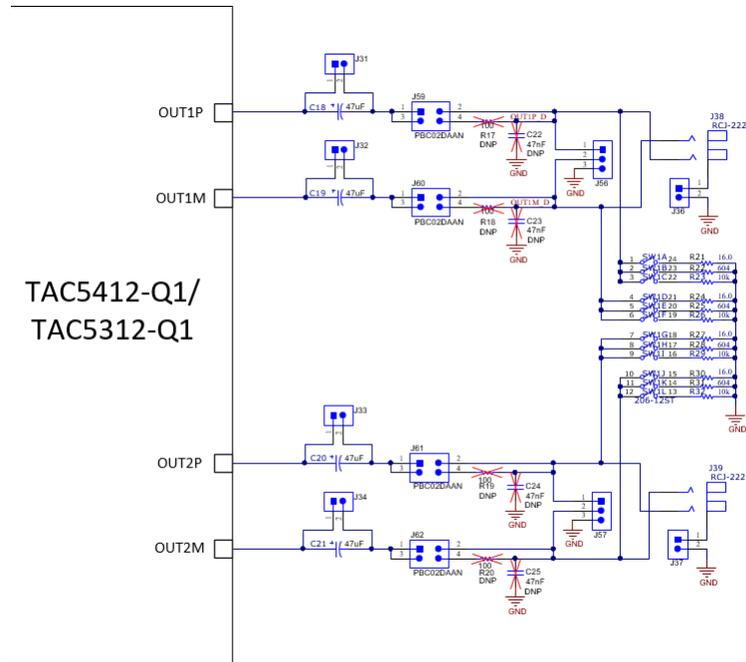
**Figure 2-12. TAC5x12-Q1 EVM Output Architecture for Channel 1 and 2**
