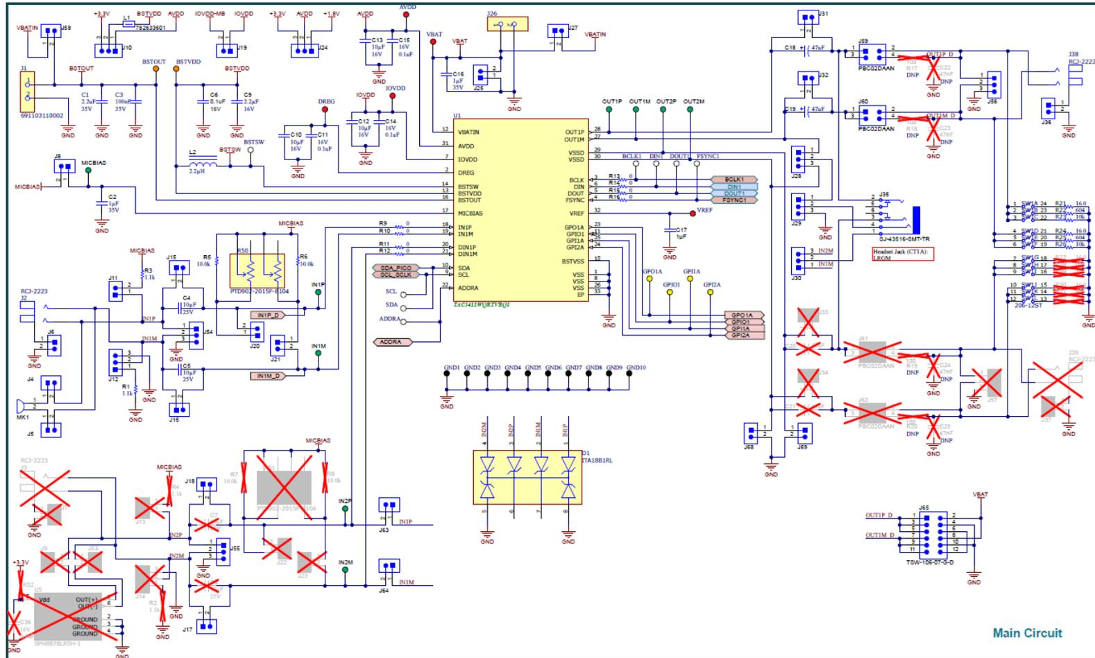
Figure 4-3. TAC5411-Q1 EVM Main DUT Schematic
