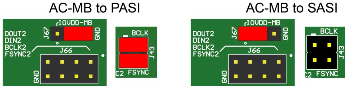
Figure 2-24. AC\_MB Audio Serial Interface Connection
