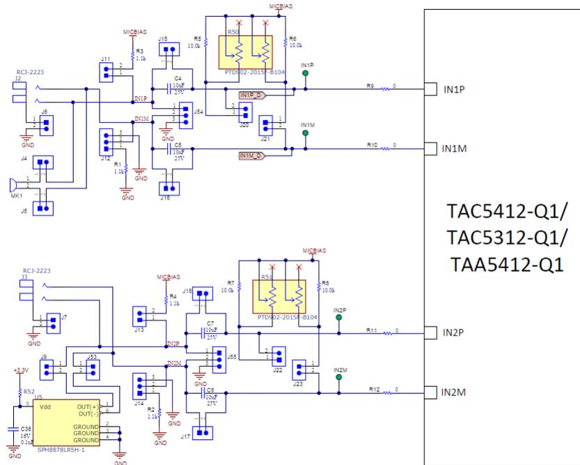
**Figure 2-9. TA5x12-Q1 EVM Input Architecture for Channel 1 and 2**
