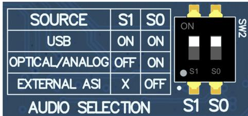
Figure 2-4. AC-MB USB Audio Setting
