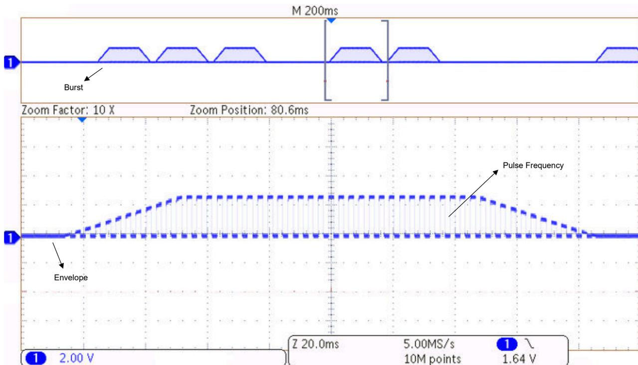
Figure 3. High Alarm State Waveform
