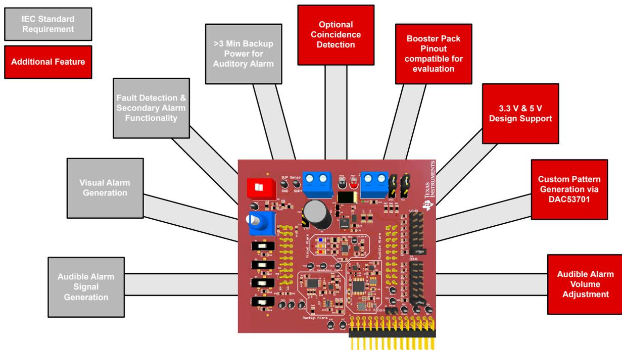
Figure 1. Medical Alarm Design using DAC53701 Smart DAC
