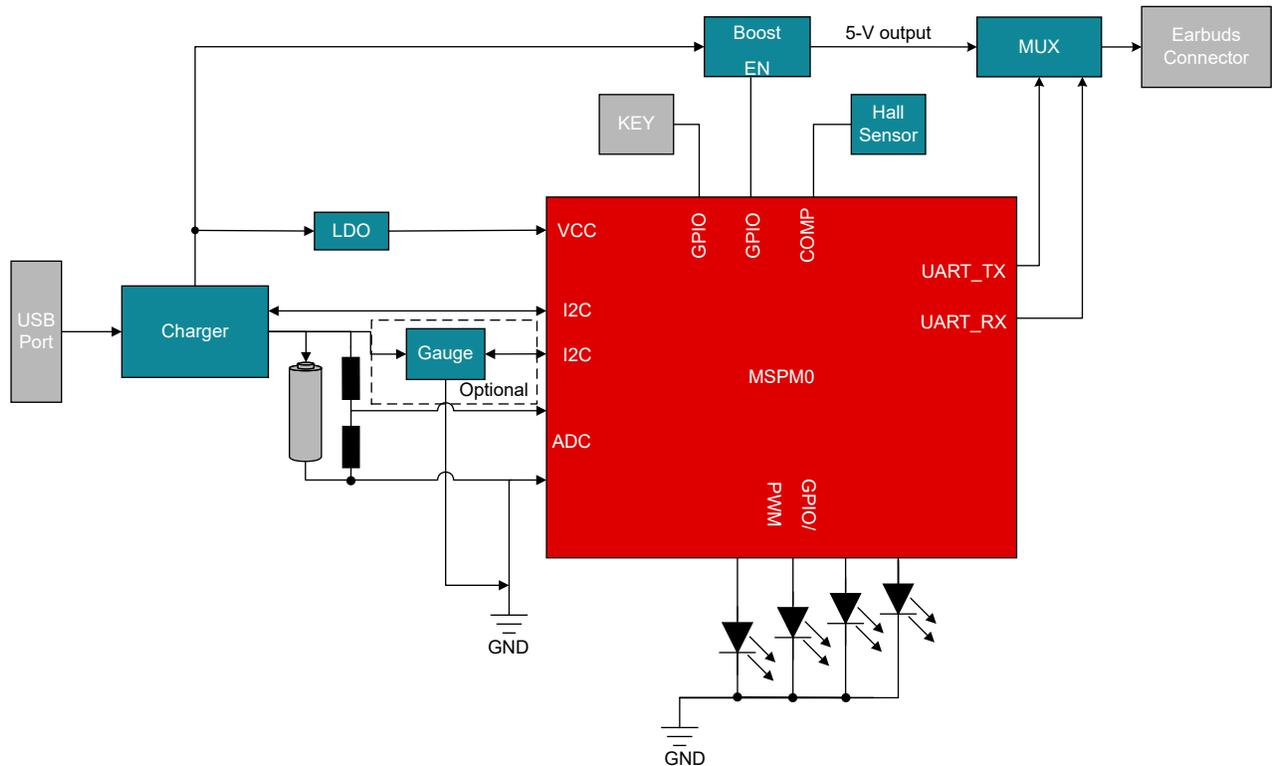
**Figure 3. Block Diagram With MSPM0 MCU**
