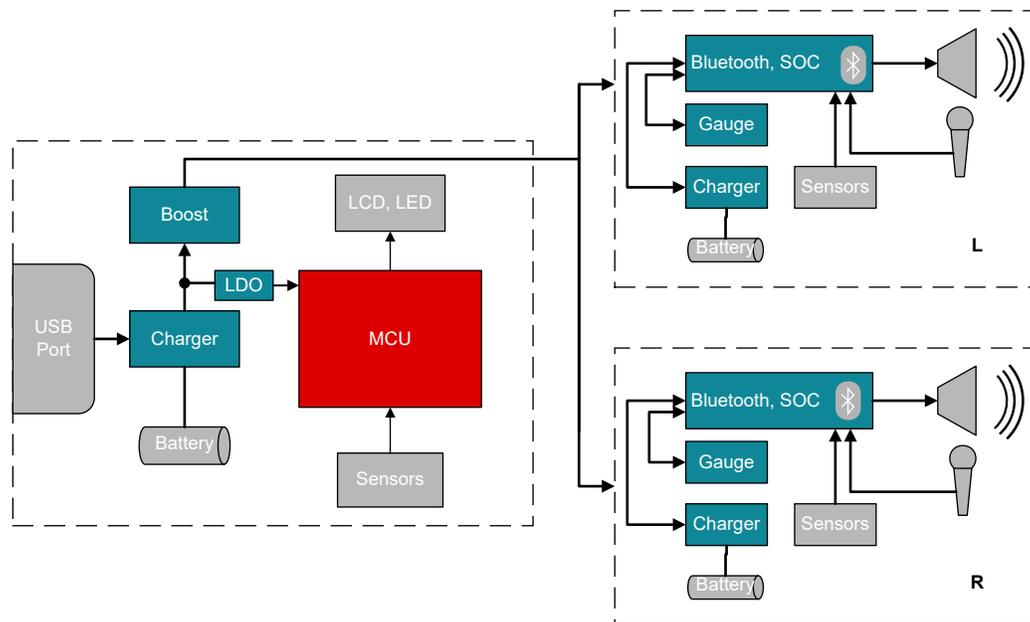
Figure 1. TWS System Block Diagram
