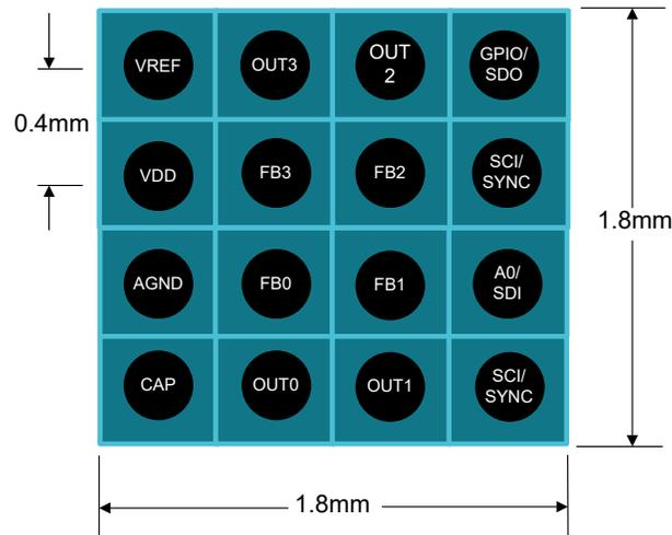
Figure 2. DACx3004W and DACx3204W Pinout
