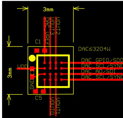
Figure 4. Typical Routing for Voltage Output
