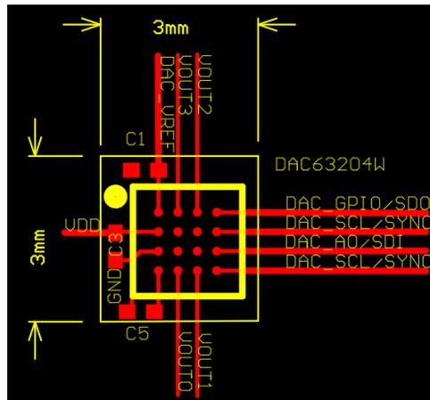
**Figure 6. Typical Routing for Current Output**
