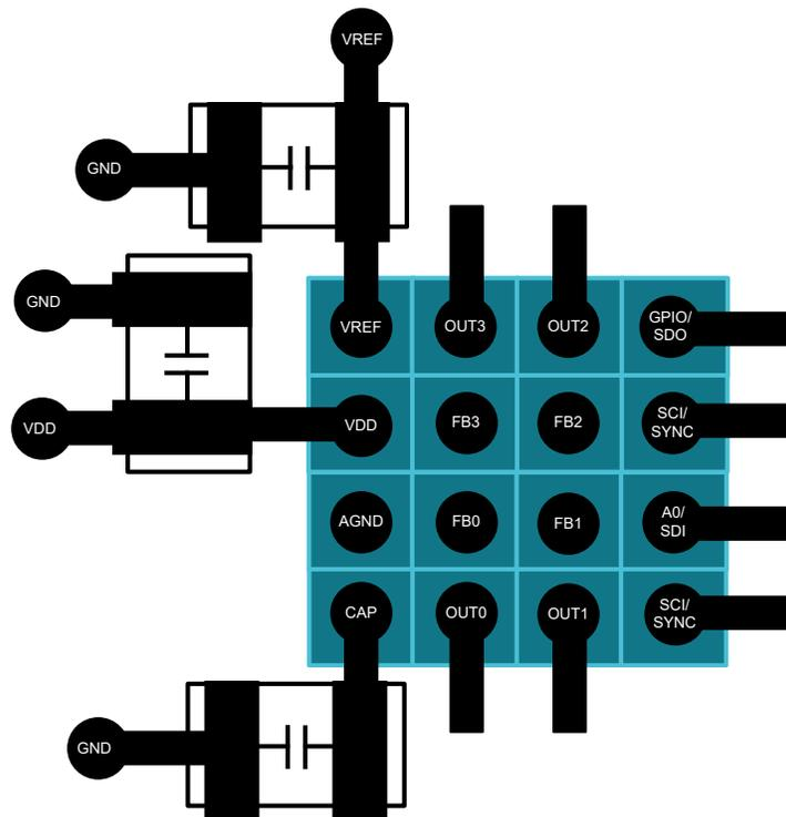
Figure 5. Current Output Configuration
