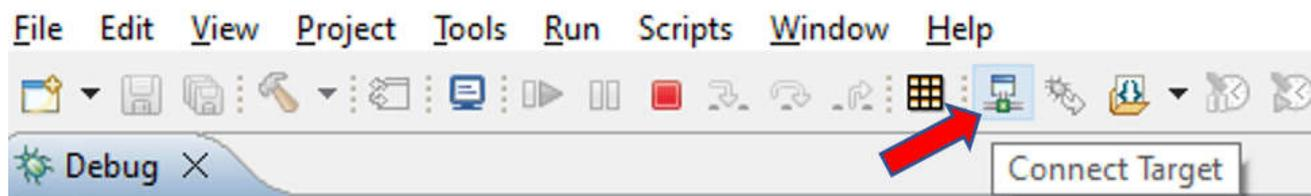
Figure 5-2. Connect the Device in CCS
