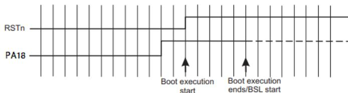
**Figure 10-1. BSL Entry Sequence at Configured GPIO Pin**
