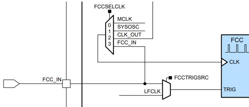
Figure 4-4. MSPM0L Series Frequency Clock Counter Block Diagram
