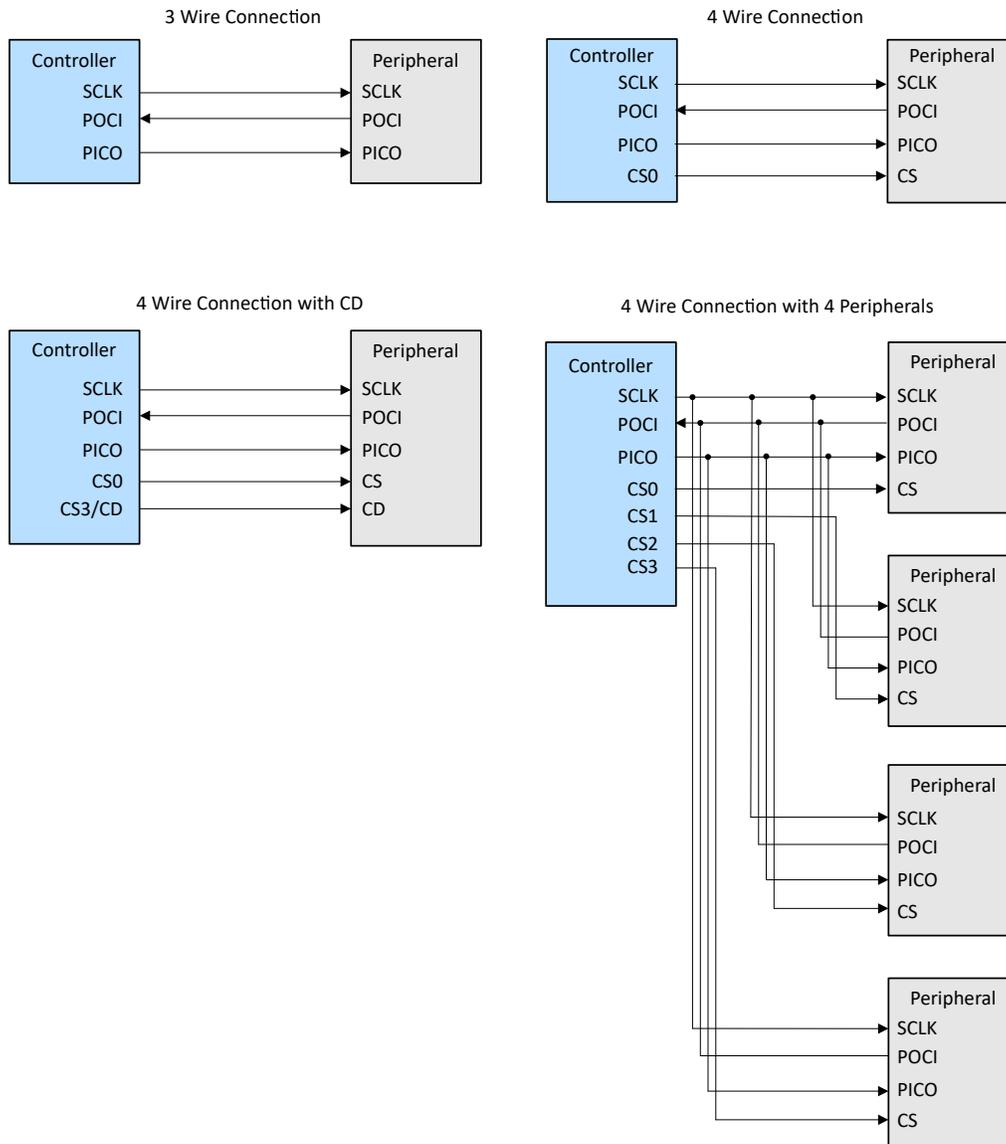
**Figure 7-4. External Connections for Different SPI Configurations**
