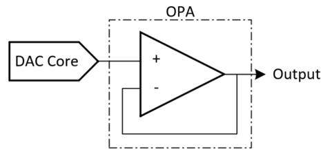
Figure 6-5. 8-Bit DAC + OPA Output Connections
