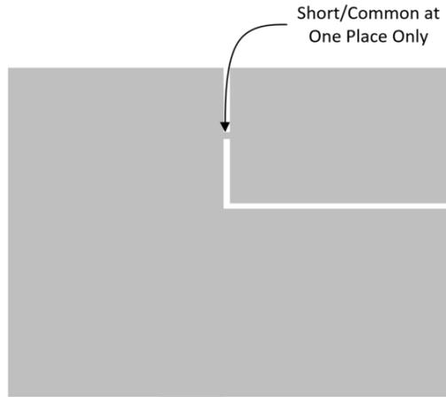
**Figure 9-2. Digital and Analog Grounds and Common Area**
