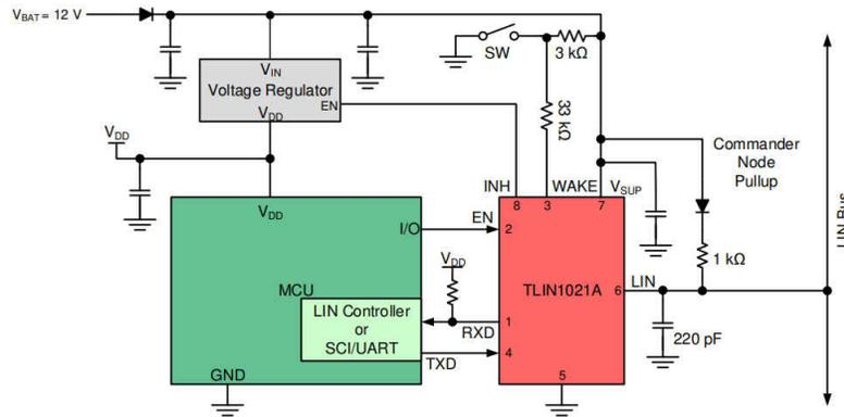
Figure 7-2. Typical LIN Application(Commander) with MSPM0L
