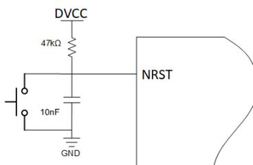
**Figure 3-1. NRST Recommended Circuit**
