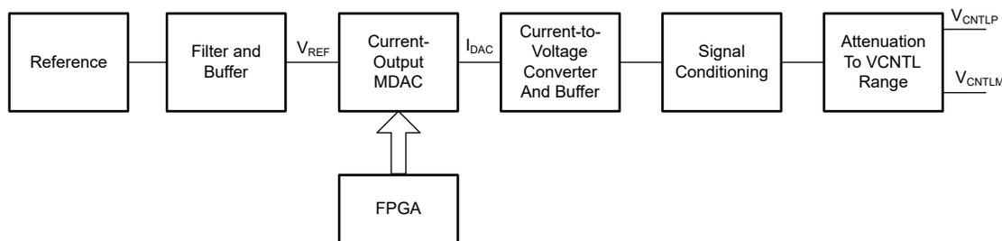
Figure 2-5. A Current-Output MDAC is Used in Generating a TGC Signal
