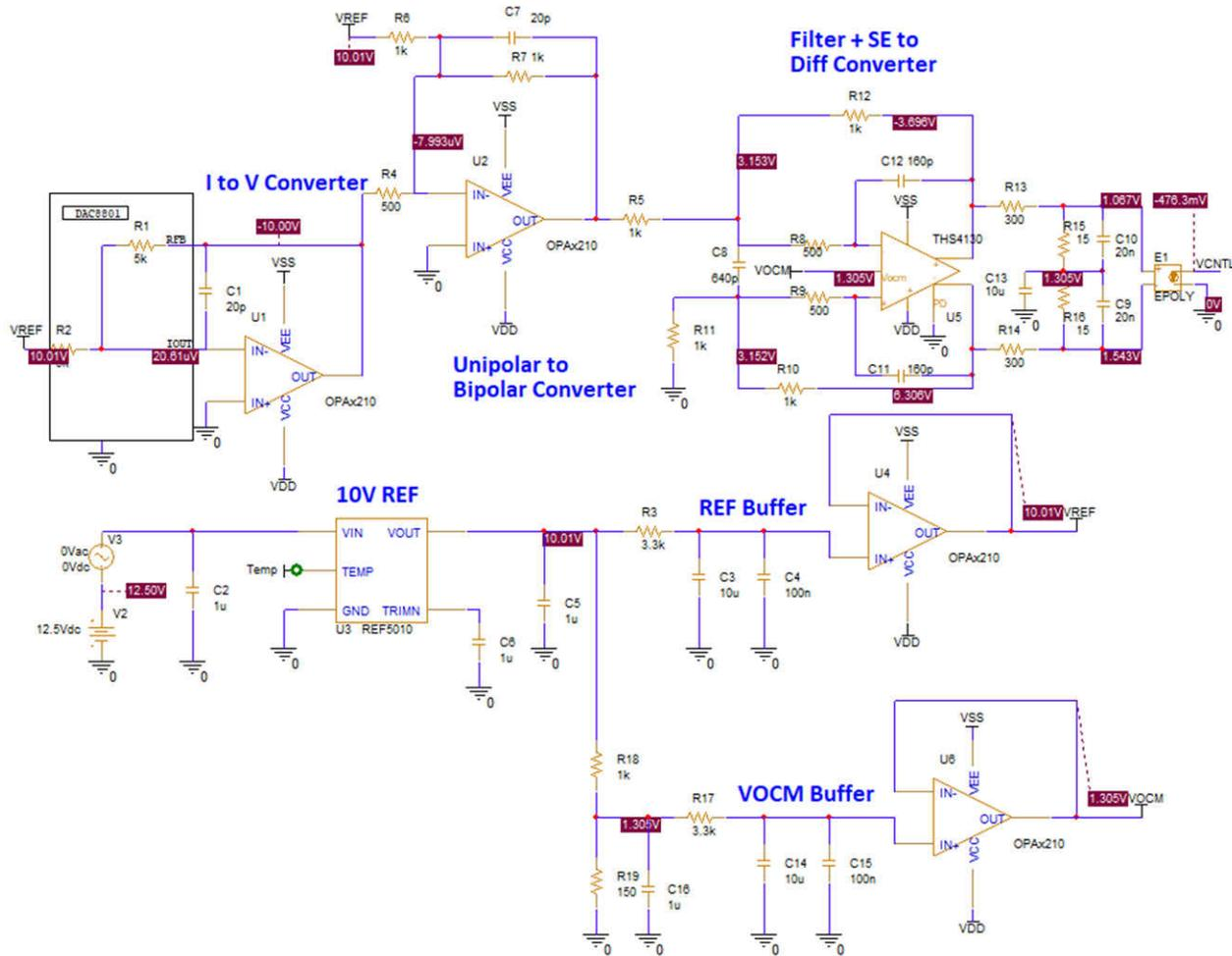
Figure 2-10. PSpice-TI Simulation of the Proposal 2  $V_{CNTL}$  Drive Circuit
