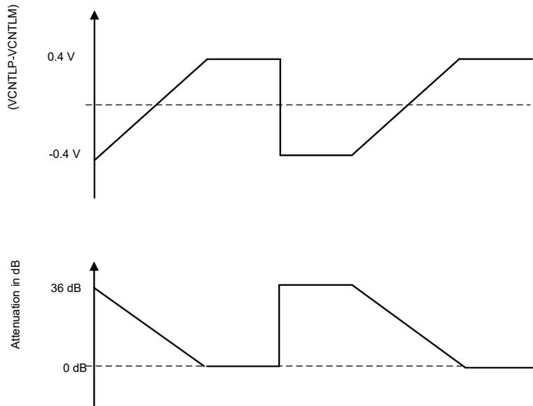
**Figure 1-2. Relationship Between  $V_{CNTL}$  Voltage and Attenuation**
