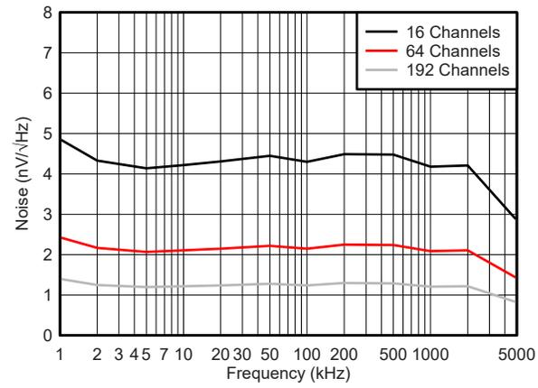
**Figure 1-4. Allowed Noise on the  $V_{CNTL}$  Signal Across Frequency and Different Channels**
