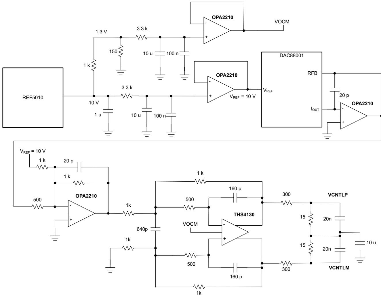
**Figure 2-6. Proposal 2  $V_{CNTL}$  Drive Circuit**
