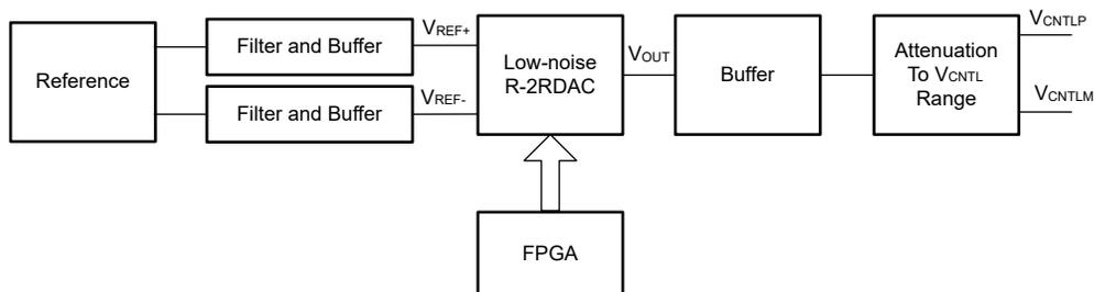
Figure 2-12. A Low-Noise R-2R DAC Used in Generating a TGC Signal
