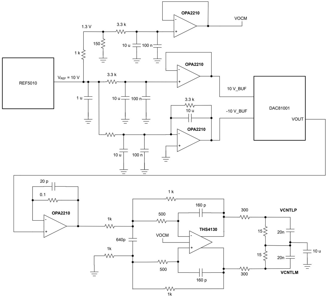
Figure 2-13. Proposal 3-V<sub>CNTL</sub> Drive Circuit
