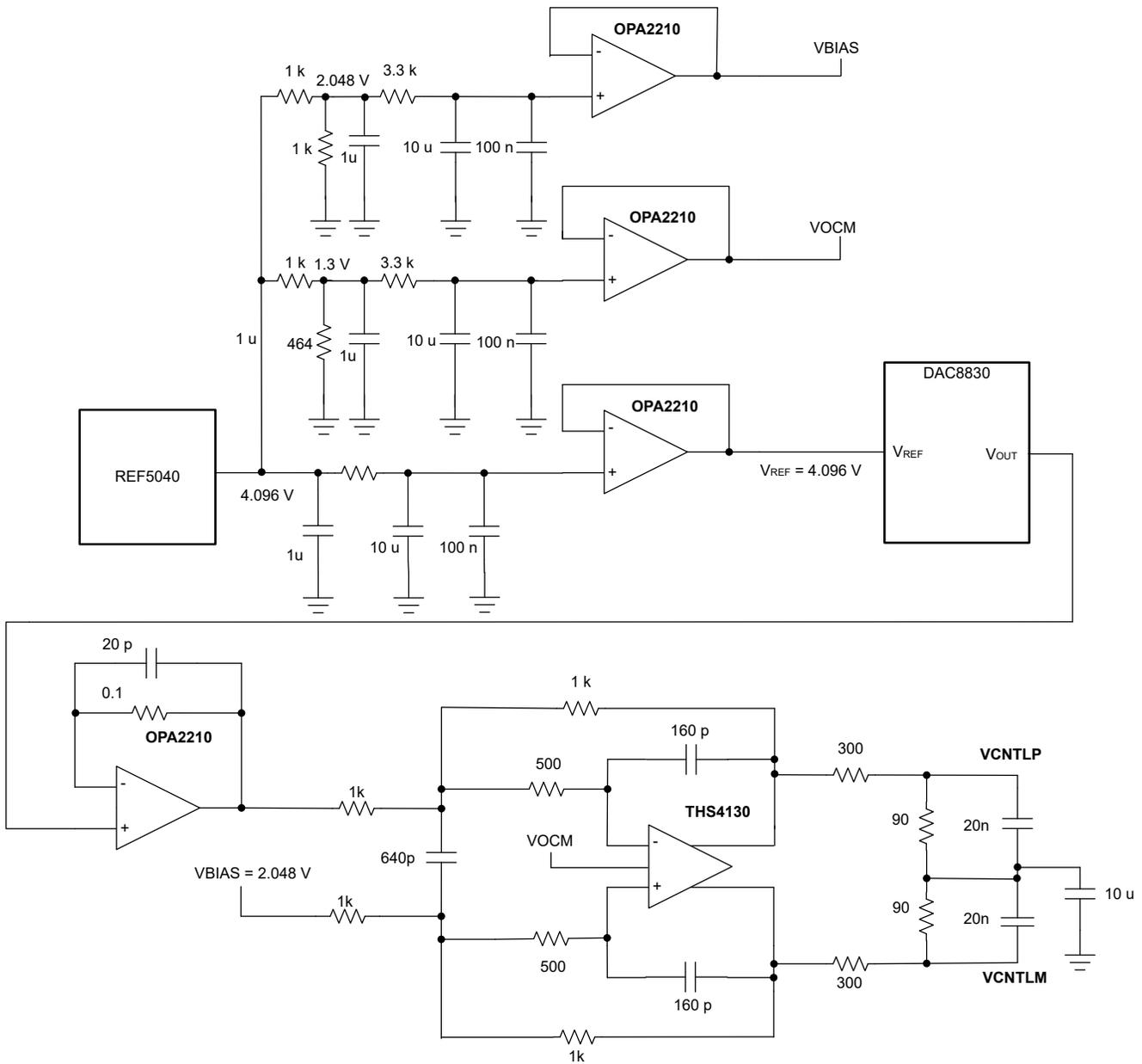
Figure 2-2. Proposal 1- $V_{CNTL}$  Drive Circuit
