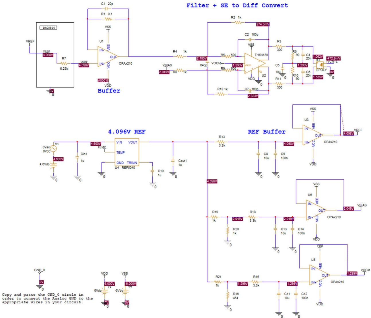
Figure 2-3. PSpice-TI Simulation of the Proposal 1 V<sub>cntl</sub> Drive Circuit
