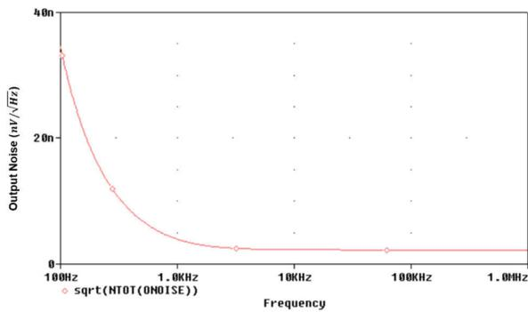
Figure 2-8. Noise Contribution From the Reference Circuit
