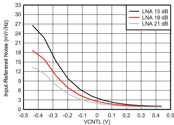
**Figure 1-3. Input-Referred Noise vs  $V_{CNTL}$  and LNA Gains for Low-Noise Mode**
