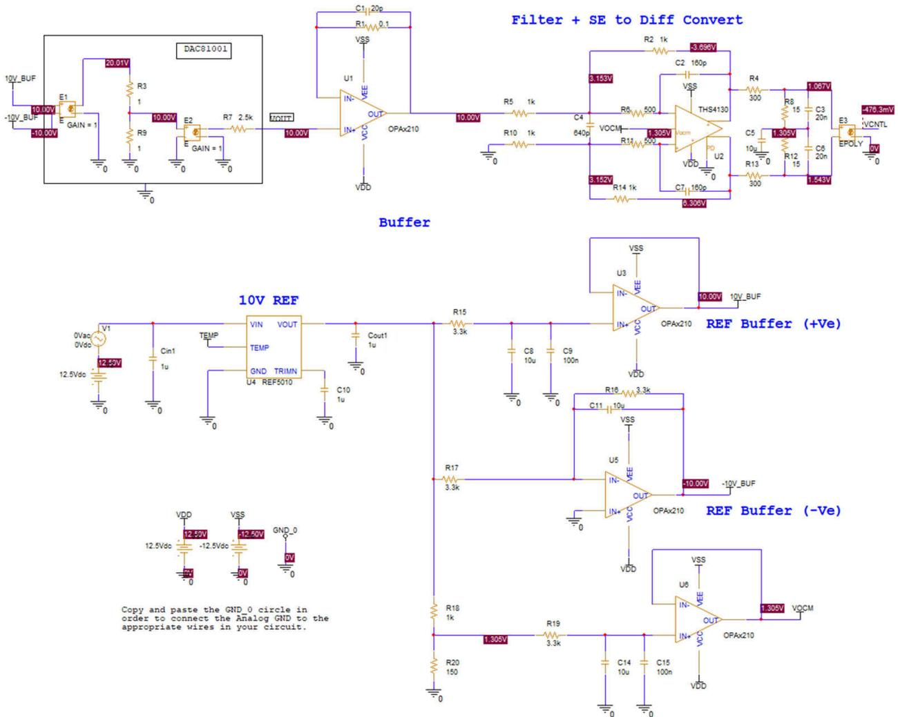
Figure 2-14. PSpice-TI Simulation of the Proposal 3- $V_{CNTL}$  Drive Circuit
