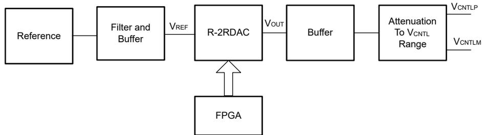
**Figure 2-1. A R-2R DAC Used in Generating a TGC Signal**
