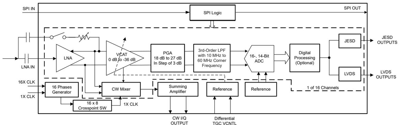
**Figure 1-1. Signal Chain of the AFE58JD48 and Analog Control for TGC Operation**
