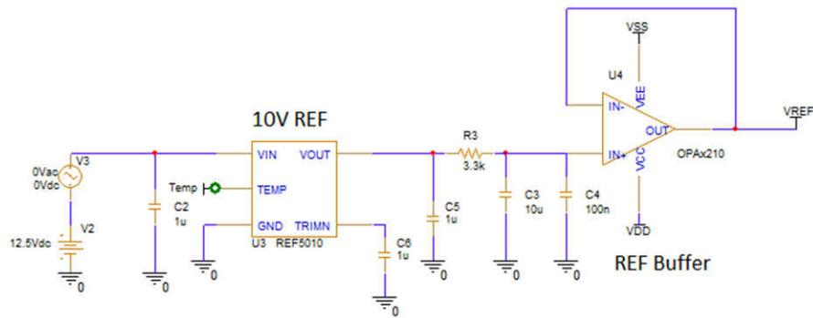
Figure 2-7. PSpice-TI Simulation for Reference Circuit (in previous image)
