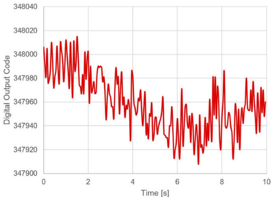
**Figure 2-7. PIR Signal Ripples/Noise**
