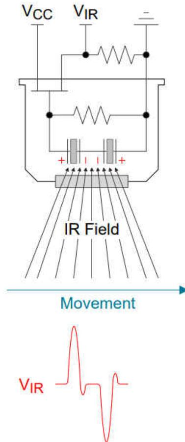
**Figure 1-2. PIR Motion Sensor Illustration**
