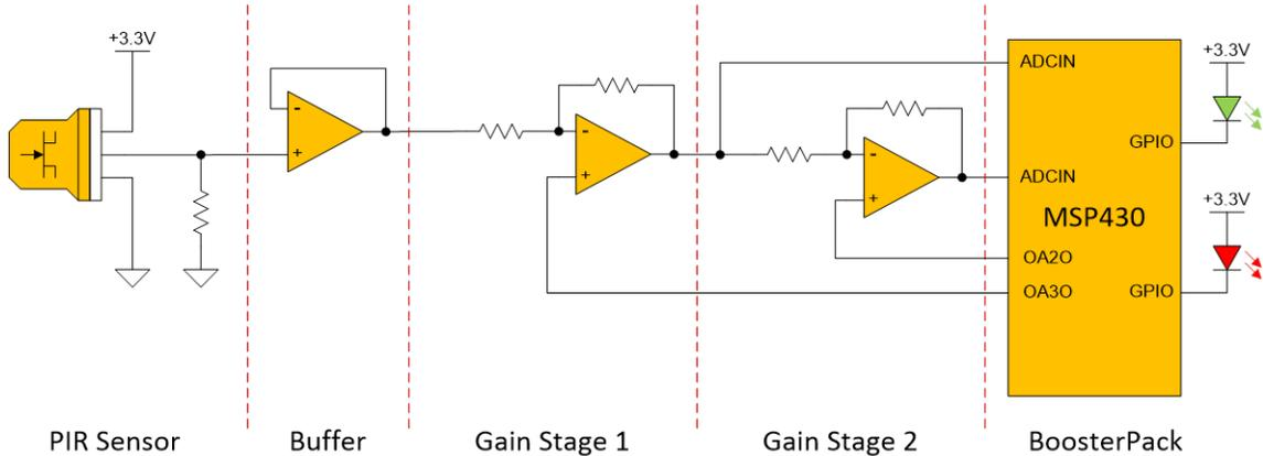
Figure 1-6. Capacitor Free Signal-Chain
