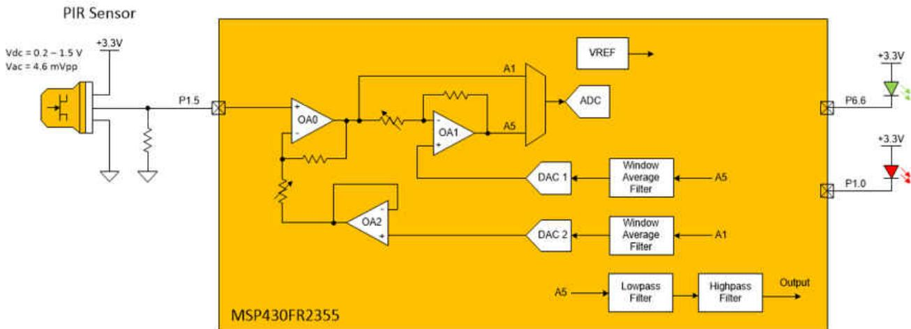
Figure 1-7. PIR Signal-Chain Integrated Into MSP430FR2355
