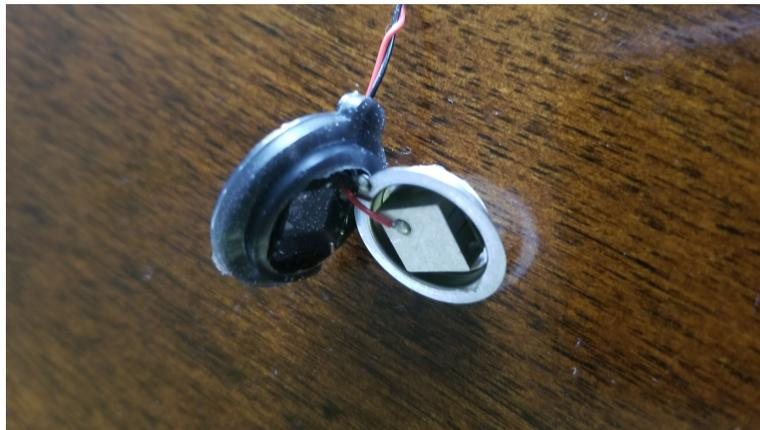
**Figure 2-2. Typical Ultrasonic Transducer Construction**
