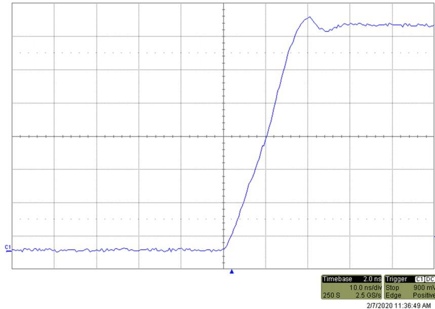
**Figure 3-4. TAS2563:  $dV/dt = 0.7 \text{ V/ns}$**
