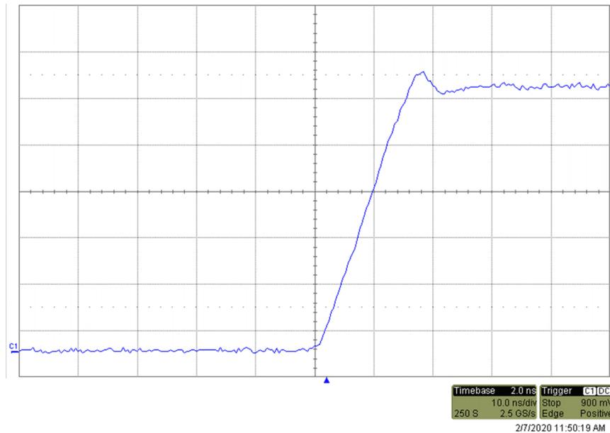
**Figure 3-2. TAS2770:  $dV/dt = 2 \text{ V/ns}$**
