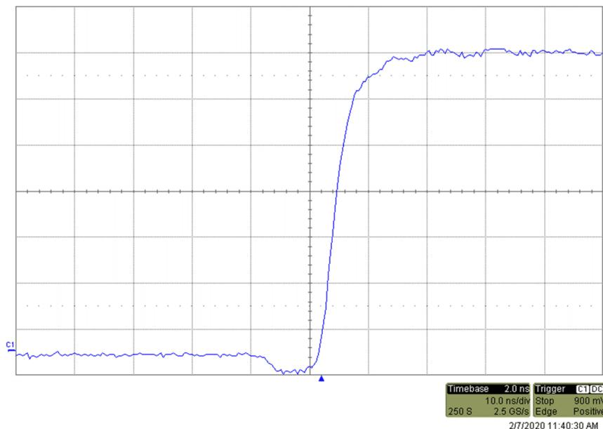
**Figure 3-5. TAS2564:  $dV/dt = 0.7 \text{ V/ns}$**
