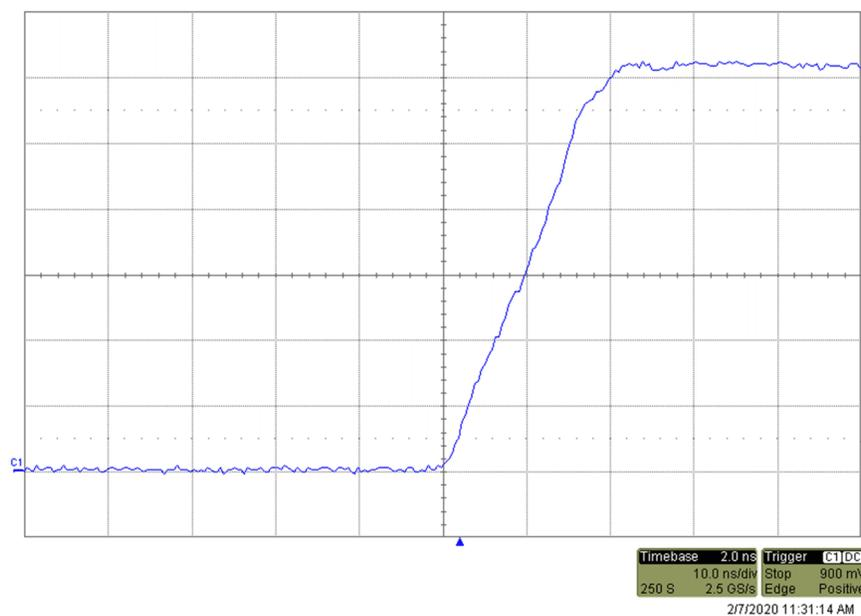
**Figure 3-3. TAS2562:  $dV/dt = 0.7 \text{ V/ns}$**
