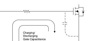
Figure 3. Explanation for MOSFET Gate Loss
