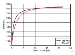
Figure 4. Efficiency vs. Output Power in Different Switching Frequency (BD Mode)
