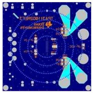
Figure 13. A Good Example of IC Placement
