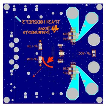
Figure 15. An Example of a Circular Cut
