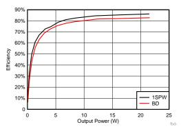
Figure 10. Efficiency vs. Output Power with Different Modulation Mode (Fsw = 768 kHz)
