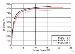
Figure 11. Efficiency vs. Output Power with Different PVDD (1SPW Mode)
