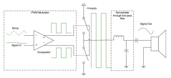
Figure 1. Typical Block Diagram of Class-D Audio Amplifier
