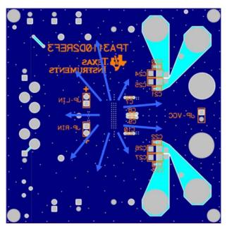
Figure 14. An Example of a Radial Cut
