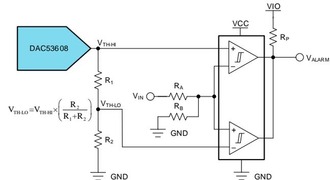
Figure 6. Resource Optimized Fault Indication
