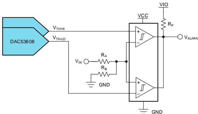
Figure 4. Window Comparator for Fault Indication
