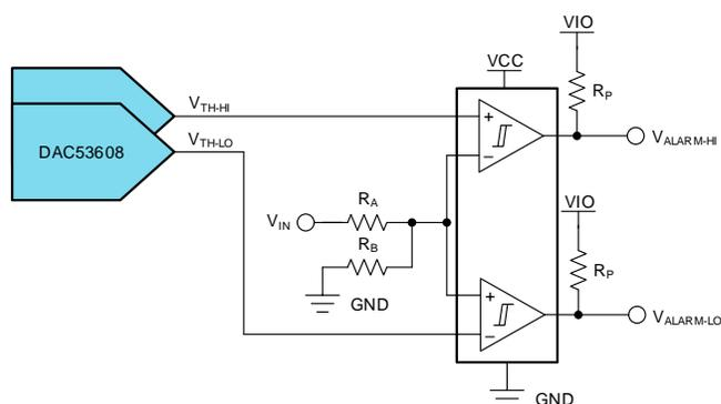
Figure 2. Window Comparator for Control Loop
