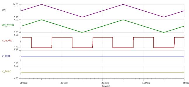
Figure 5. Fault Indication Waveform
