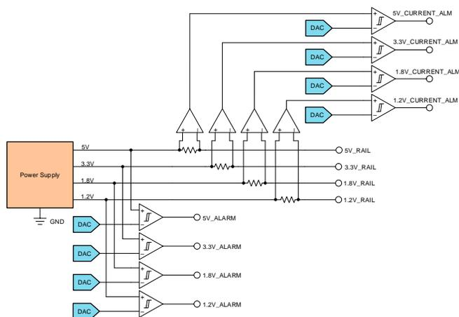
Figure 1. Block Diagram of Power Supply Supervision
