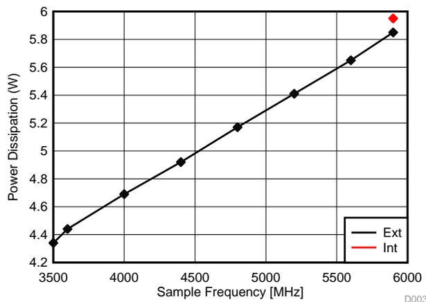
Figure 3. Power Dissipation vs. External Sample Clock
