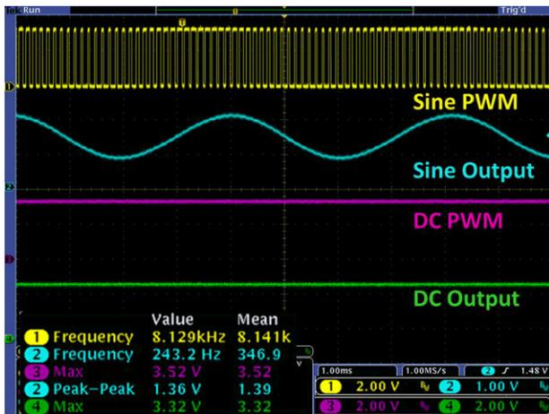
Figure 4. C2 = 420 pF, 3.32 VDC, 100% PWM
