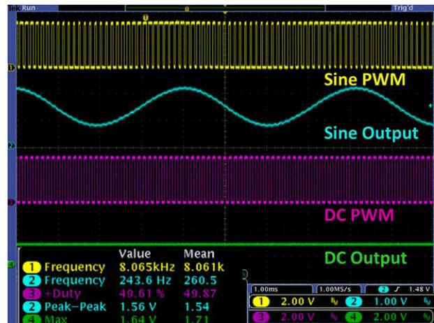
Figure 3. C2 = 220 pF, 1.64 VDC, 50% PWM
