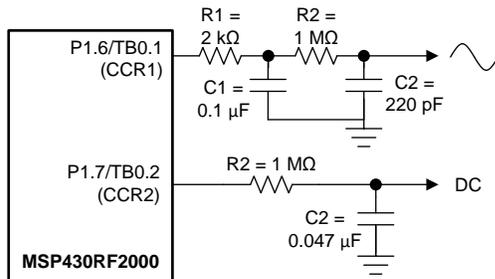
Figure 2. Output Filter Diagram
