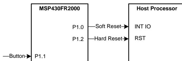
**Figure 1. Reset Controller Block Diagram**
