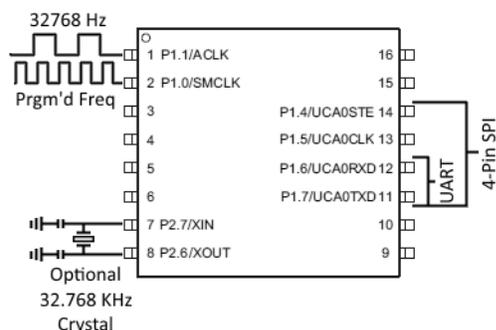
**Figure 1. Programmable Clock Source Inputs/Outputs**
