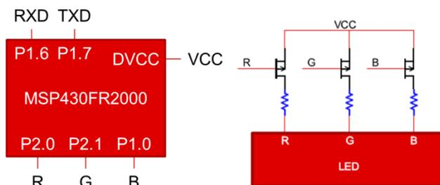
Figure 1. RGB LED Controller Block Diagram
