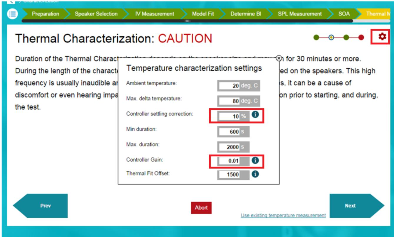
The screenshot shows the 'Thermal Characterization: CAUTION' settings panel. The top navigation bar includes steps: Preparation, Speaker Selection, IV Measurement, Model Fit, Determine BI, SPL Measurement, SOA, and Thermal M. The main panel contains the following settings:
