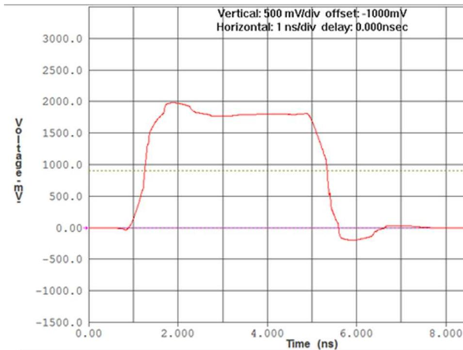
Figure 12. Signal at Driver Load – HyperLynx
