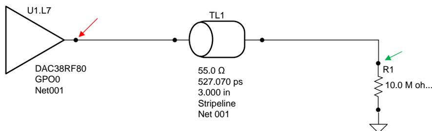
Figure 9. Signal Integrity Simulation Circuit – HyperLynx
