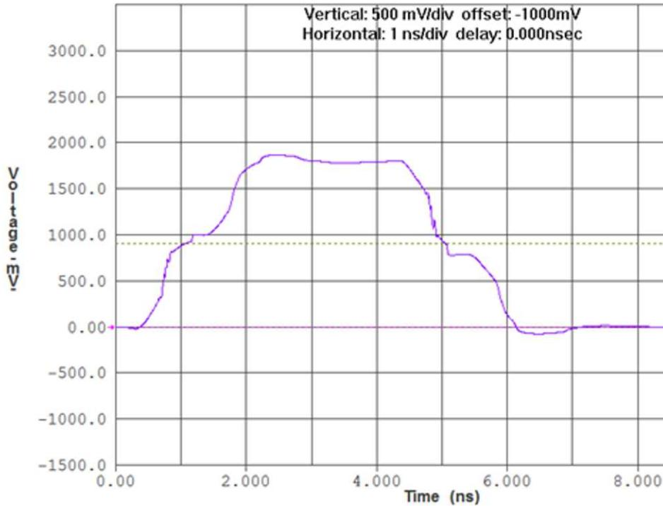
Figure 11. Signal at Driver Pin – HyperLynx
