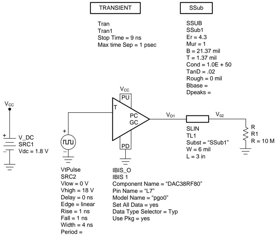
Figure 5. Signal Integrity Simulation Circuit – ADS
