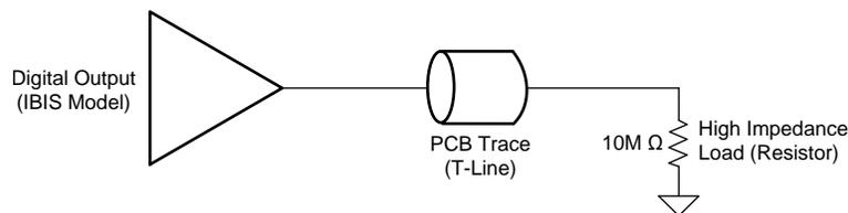
**Figure 1. ADS and HyperLynx Simulated Circuit**
