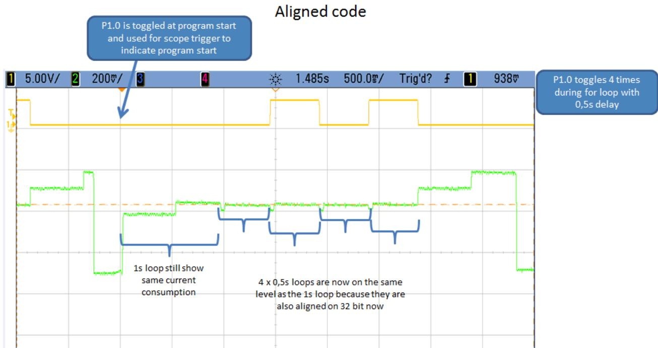
Figure 8. Manual Code Alignment to 32 Bit
