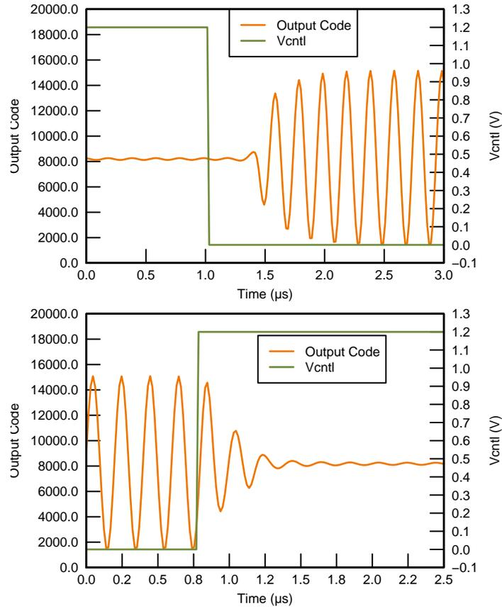
Figure 8. Control Voltage and Settling Time Relationships
