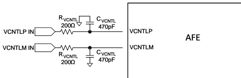
Figure 7. Filtering on  $V_{CNTLx}$  Pins
