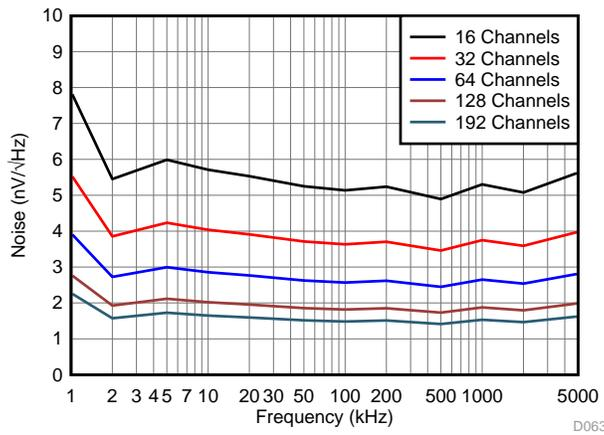
Figure 6. Allowed Noise on the  $V_{CNTL}$  Signal Across Frequency and Different Channels
