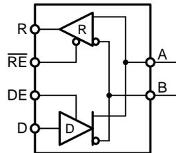
**Figure 1. Block Diagram of a Half Duplex RS-485 Transceiver**
