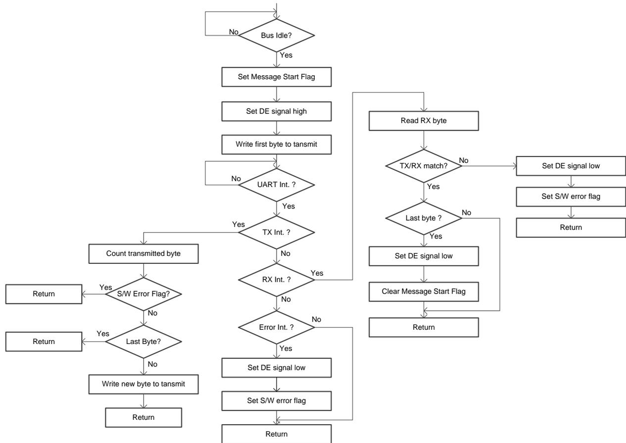
Figure 2. Process of Sending a RS-485 Message
