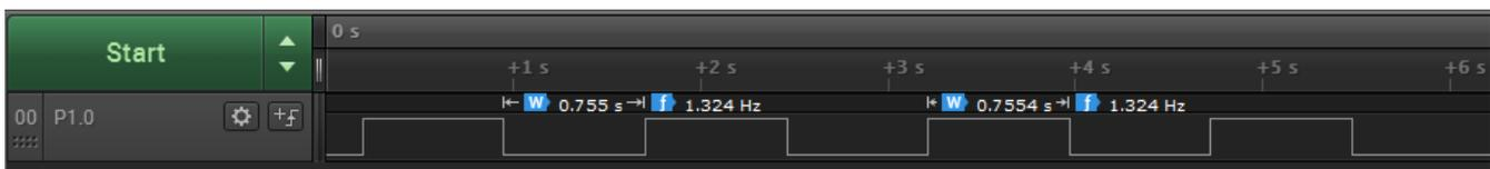
Figure 5. RTC Timing Without VLO Calibration
