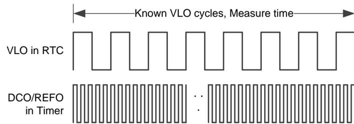
**Figure 1. VLO Frequency Measurement Method 1**
