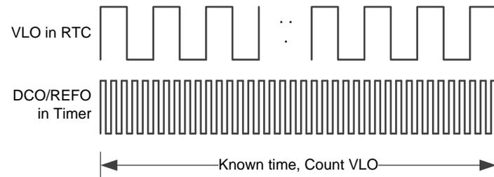
**Figure 2. VLO Frequency Measurement Method 2**
