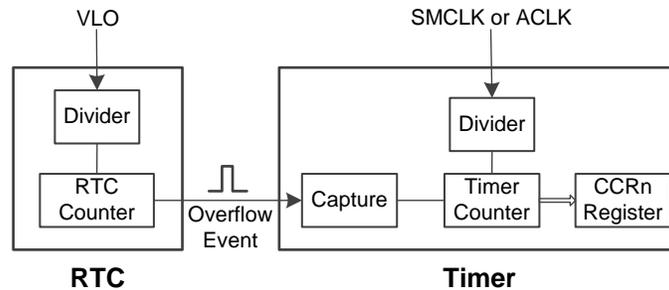
**Figure 3. Peripherals Used for VLO Calibration**
