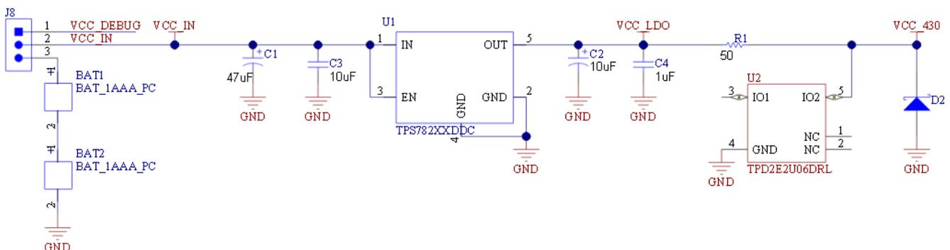
**Figure 3-6. Alternative Solution Using a Zener Diode**
