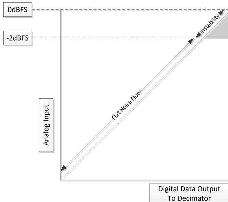
**Figure 2. Input vs Output graph of a Delta Sigma Modulator**
