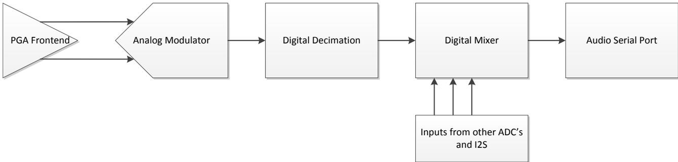
**Figure 1. ADC Signal Chain Architecture of PCM186x**
