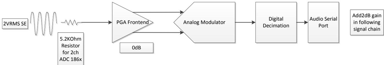
**Figure 4. HW Controlled Compensation to Ensure 2.1 VRMS Inputs Avoid Noise Modulation**
