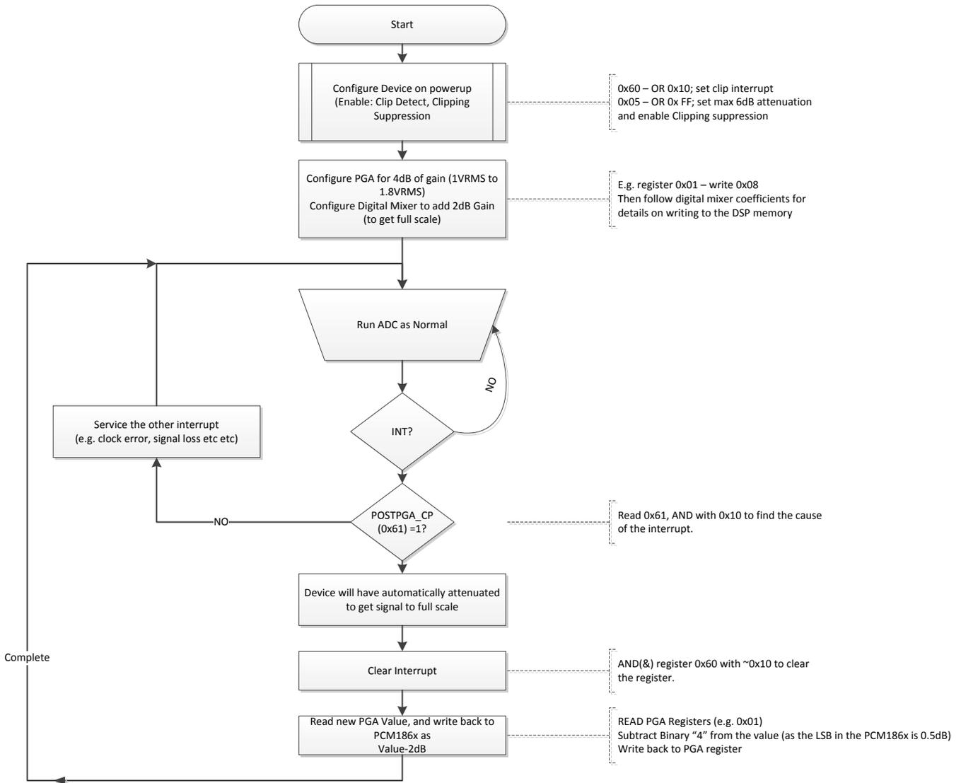
Figure 5. Workflow to Use Auto Gain Suppression With a -2 dBFS Input Signal
