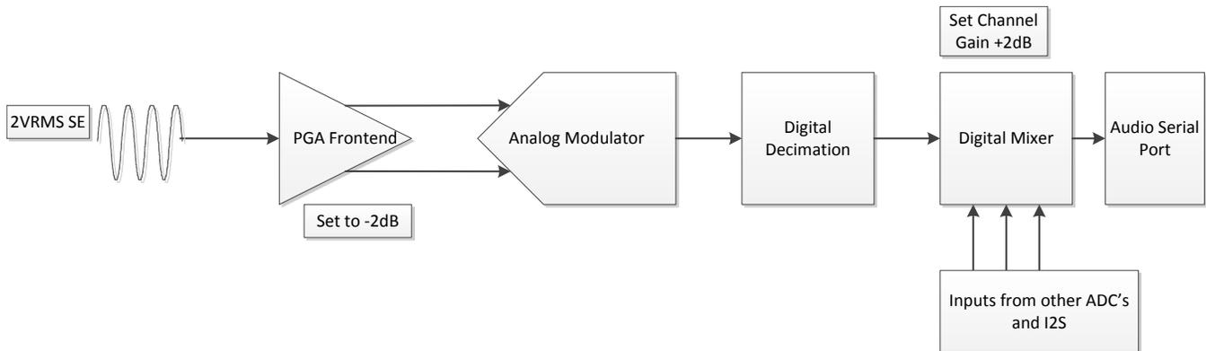
Figure 3. SW Controlled Compensation to Ensure 2.1 VRMS Inputs Avoid Noise Modulation
