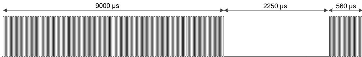
Figure 14. Pulse Distance Protocol, Repeat Frame Format
