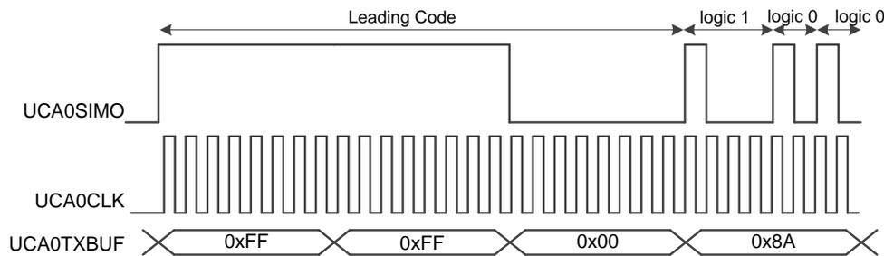
**Figure 17. Pulse Distance Protocol, SPI in Envelope Generation**
