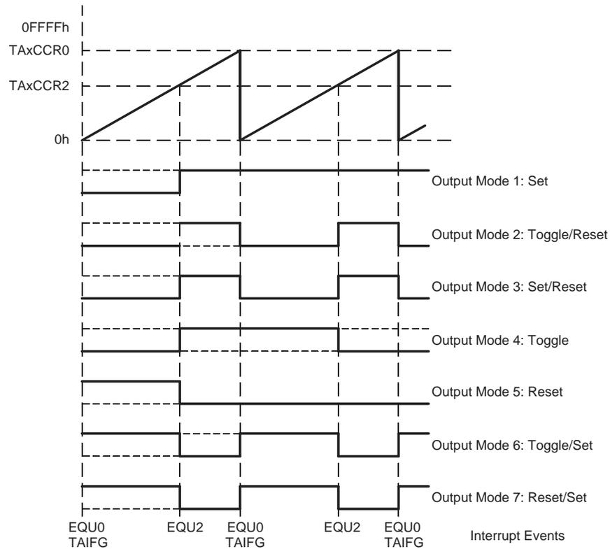
Figure 10. Output Example – Timer in Up Mode
