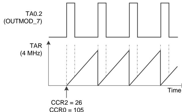
**Figure 18. Pulse Distance Protocol, TA0 in Carrier Generation**
