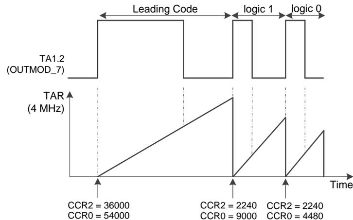
**Figure 16. Pulse Distance Protocol, TA1 in Envelope Generation**
