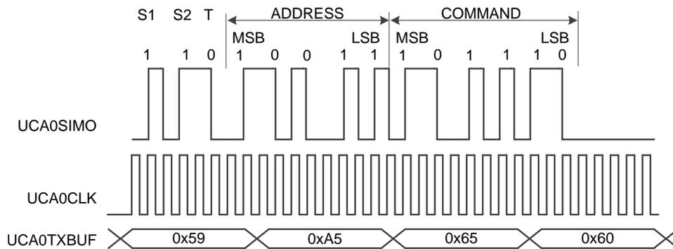
Figure 23. RC5 Protocol, SPI in Envelope Generation
