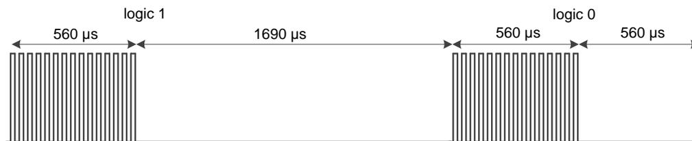
Figure 12. Pulse Distance Protocol, Bit Encoding
