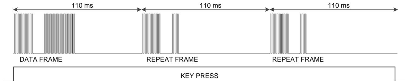
Figure 15. Pulse Distance Protocol, Full Sequence Format
