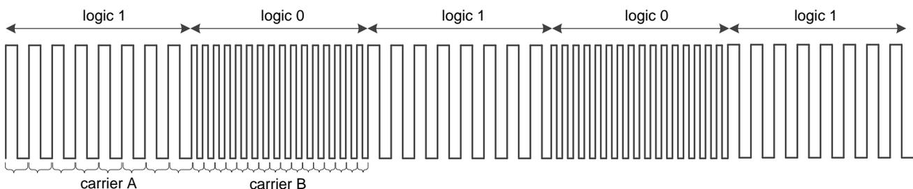
Figure 6. FSK Modulation
