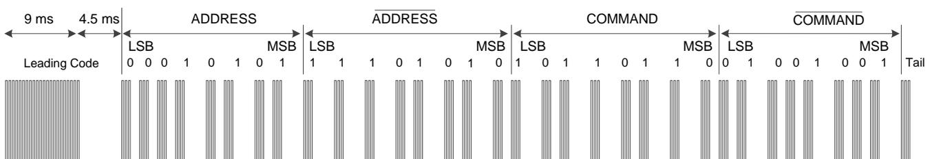
Figure 13. Pulse Distance Protocol, Data Frame Format
