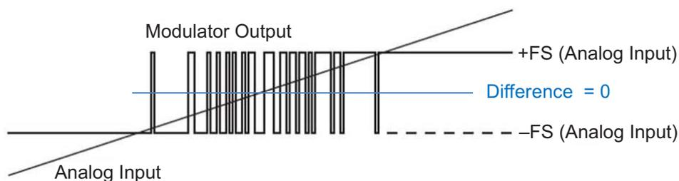
**Figure 3. Analog Input versus Modulator Output <sup>(1)</sup>**
