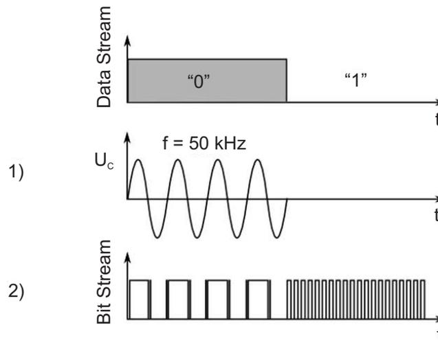
Figure 4. Expected Bit Stream from the AMC Modulator
