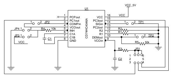
Figure 6. Typical Demodulator Schematic
