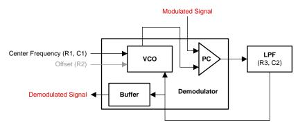
Figure 5. Basic Block Diagram of PLL as Demodulator
