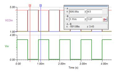
Figure 10. Simulated Waveforms of Level-Shifter Circuit using LP211
