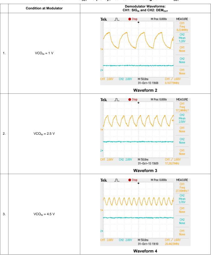
Table 3. Variation in VCO<sub>OUT</sub> Frequency, Peak-to-Peak Voltage and DEM<sub>OUT</sub>
