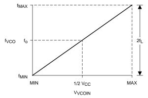
$2f_L$  = Frequency Lock Range,  $f_o$ = Center Frequency
