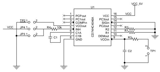
Figure 4. Typical Modulator Schematic
