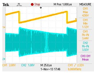
Waveform 1. VCO<sub>IN</sub> (CH1) Voltage and VCO<sub>OUT</sub> Peak-to-Peak (CH2) Variation
