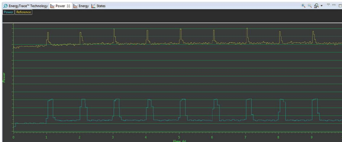
**Figure 27. MostEfficient.c Power Referenced With Inefficient.c Power**
