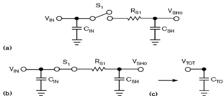
**Figure 4. Simplified Model for First-Order RC Filter**
