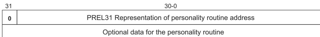
The format of the optional data is up to the discretion of the personality routine, but the length must be an integer multiple of whole 32-bit words. The unwinder calls the personality routine, passing it a pointer to the first word of optional data.
