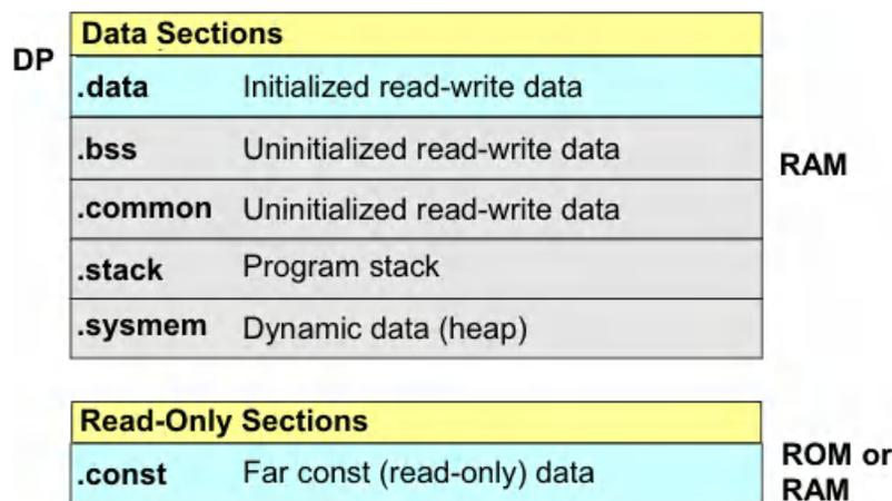
**Figure 4-1. Data Sections and Segments (Typical)**
