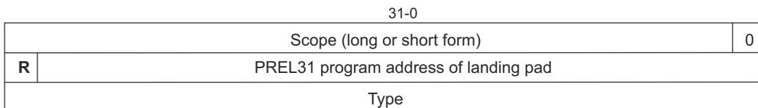
If bit R is 1, the type of the catch clause is a reference type represented by TYPE. If bit R is 0, the type is not a reference type.
