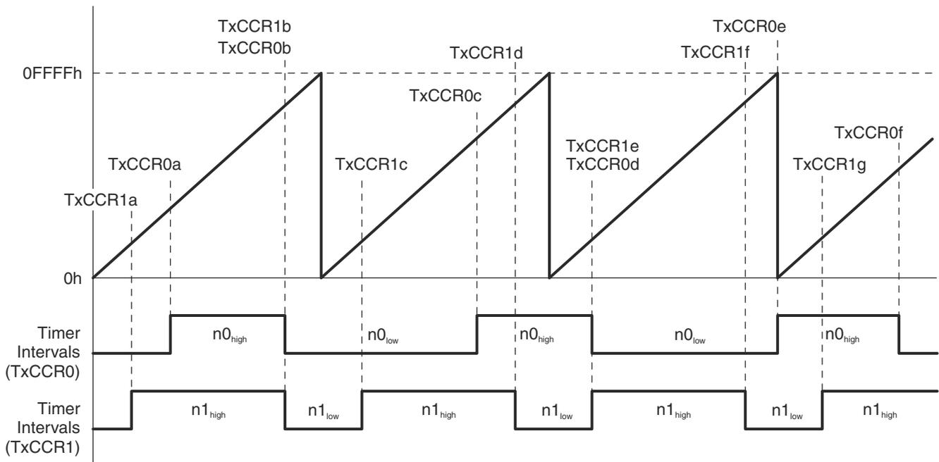
**Figure 3-1. Continuous Mode PWM Generation**
