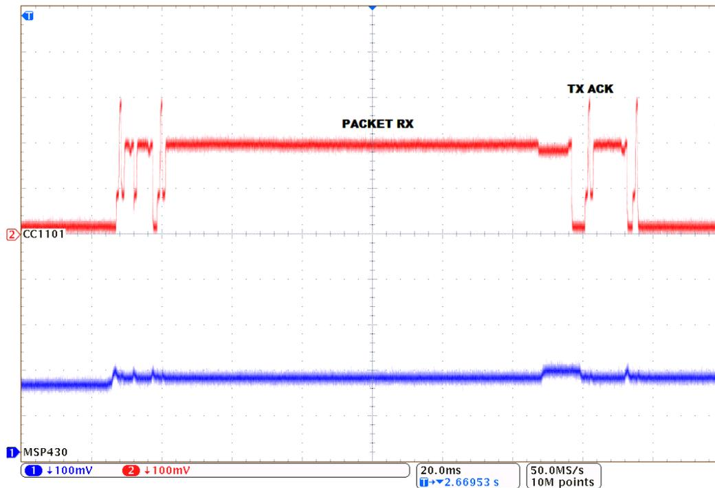
Figure 43. Current Measurement of the First Firmware Packet
