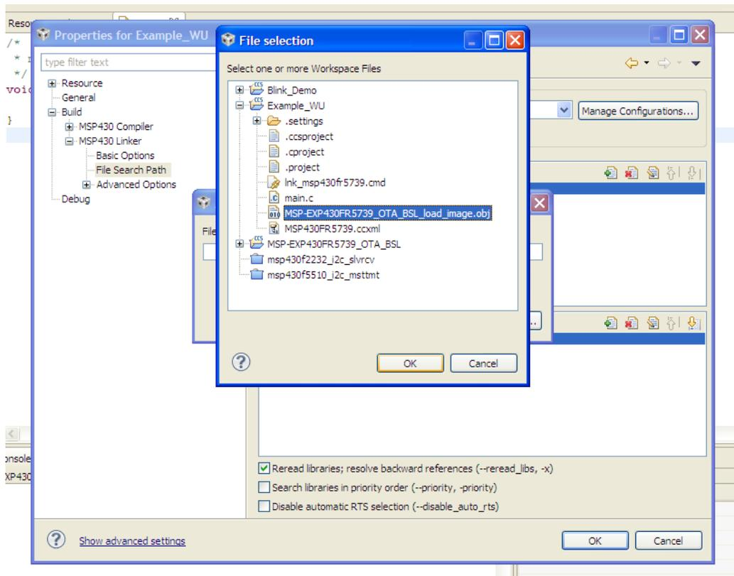
Figure 28. Include Load Image in CCS Project
