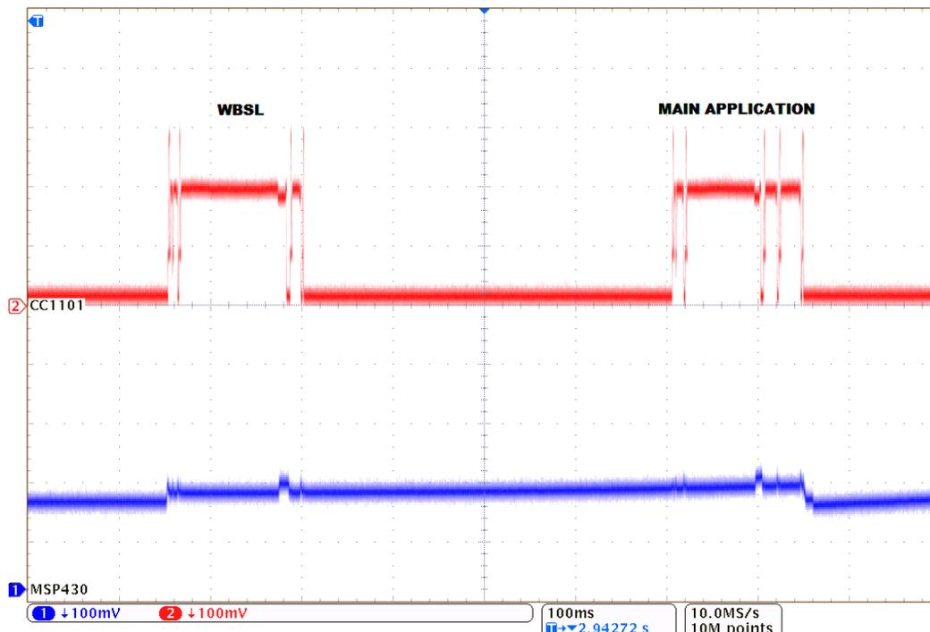
Figure 38. Current Measurement of a Wireless Update
