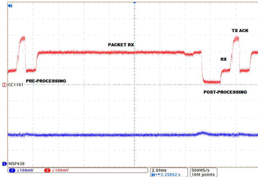
**Figure 39. Current Measurement of a Packet Transmission**
