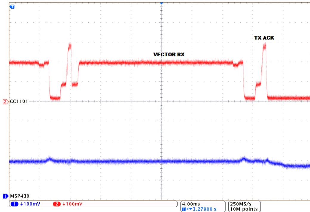
**Figure 44. Current Measurement of a Reset Vector Packet**
