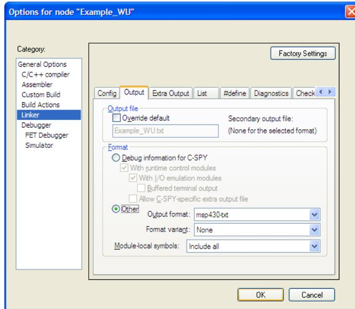
**Figure 36. Linker Output File Selection in IAR EW**
