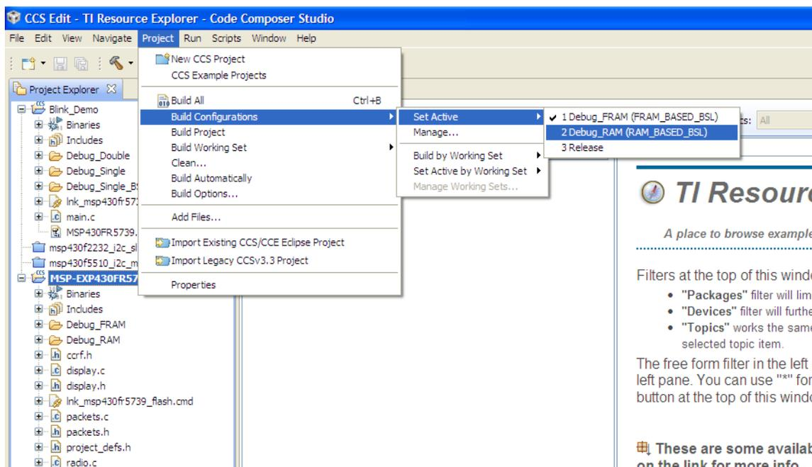
Figure 18. Code Composer Studio v5 Build Configuration Selection
