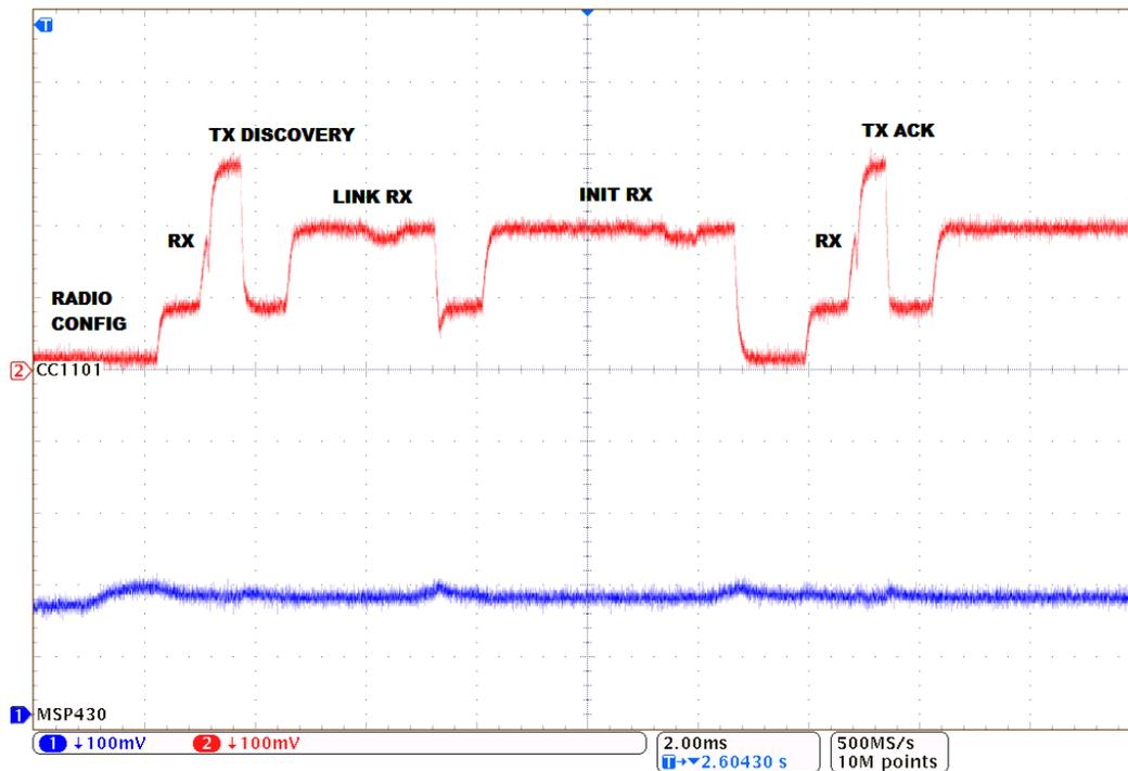
Figure 41. Current Measurement of a Link Event
