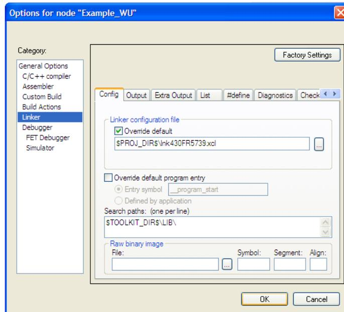
**Figure 37. Linker Configuration File Override in IAR EW**
