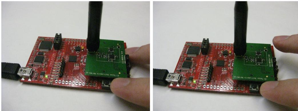
Figure 9. Hardware Initialization Sequence for Wireless Update
