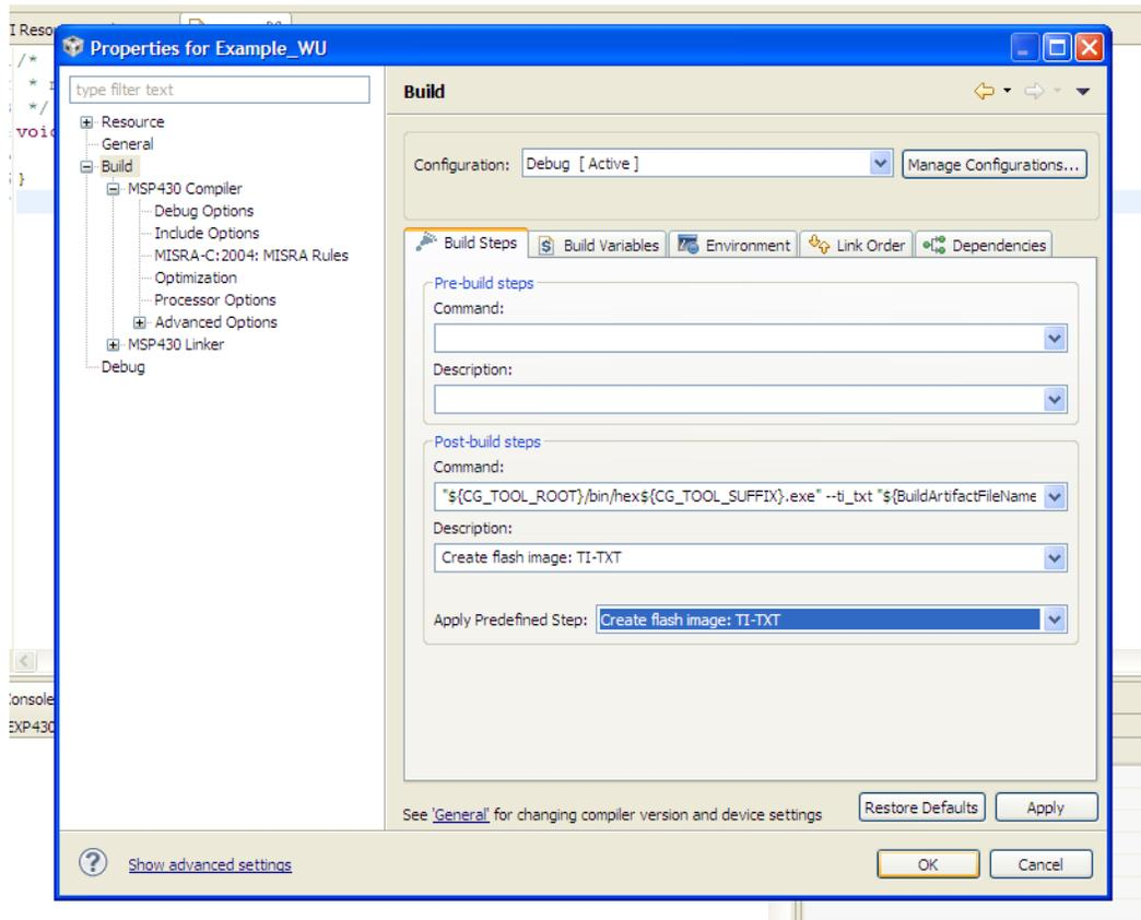
**Figure 29. Post Build Step in CCS Project**
