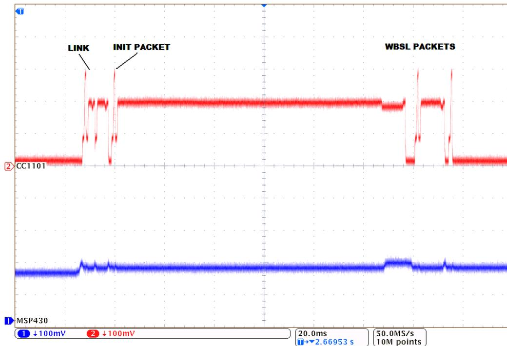
Figure 42. Current Measurement of a WBSL Transmission
