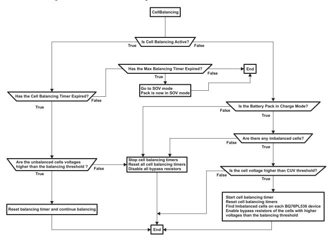
Figure 6. Cell Balancing Flowchart
