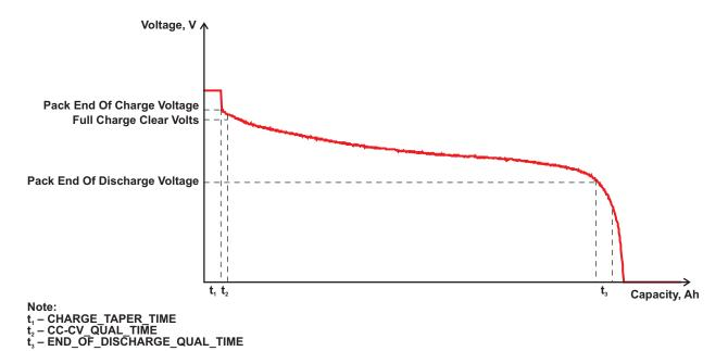
Figure 5. Battery Pack Threshold Values
