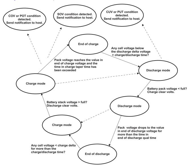
Figure 3. Battery Manager State Machine
