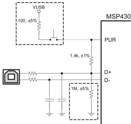
**Figure 3. Example Circuit for Hardware Invocation Circuit**
