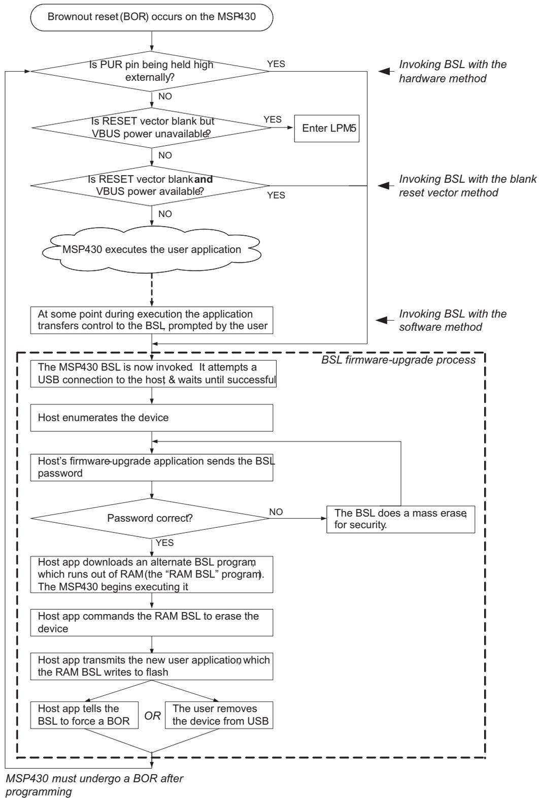
Figure 2. System-Level Description of MSP430 USB Firmware Updates
