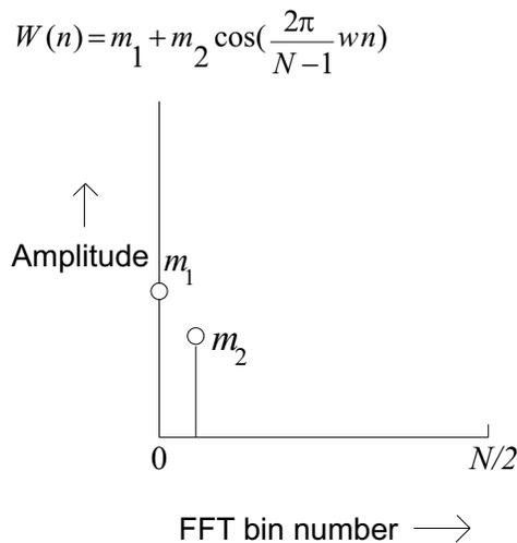
**Figure 7. Spectrum of Window Function**
