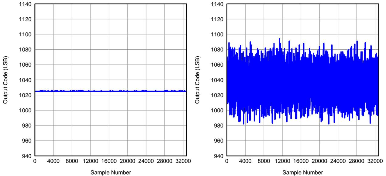
**Figure 3. Time Domain Data With SNRBoost<sup>3G</sup> Disabled and Enabled (With No Input Signal)**
