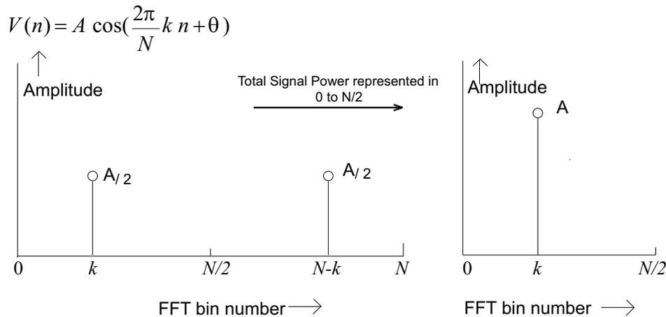
**Figure 6. Spectrum of ADC Output Sequence**
