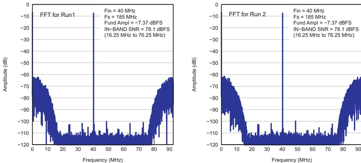
**Figure 5. Stable Spectrum With SNRBoost<sup>3G</sup> Enabled and After Windowing**
