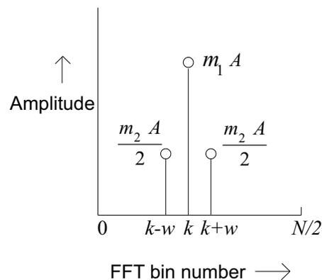
**Figure 8. Spectrum of Signal After Windowing**
