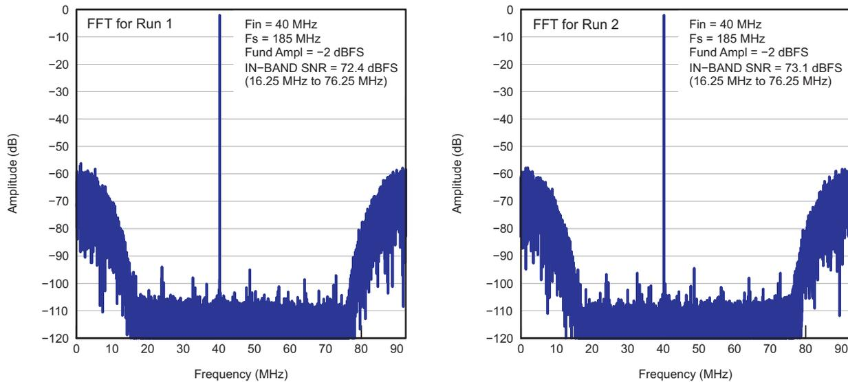
**Figure 4. Unstable Spectrum With SNRBoost<sup>3G</sup> Enabled**
