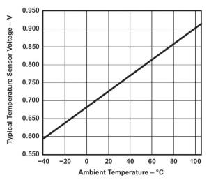
Figure 8. Typical Temperature Sensor Transfer Function
