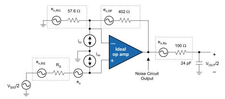
Figure 14. Noise Analysis Circuit
