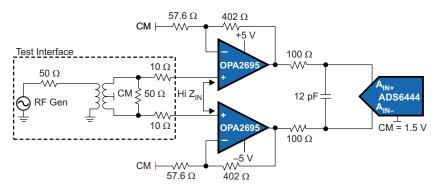
Figure 18. High-Speed, ADC Driver Amplifier with High-Impedance Inputs (Based on the OPA2695)
