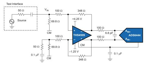
Figure 19. High-Speed ADC Driver Amplifier (Based on the THS4509)
