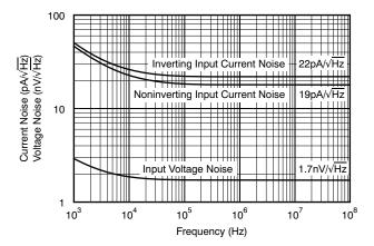
Figure 11. Input-Referred Noise for the OPA2695
