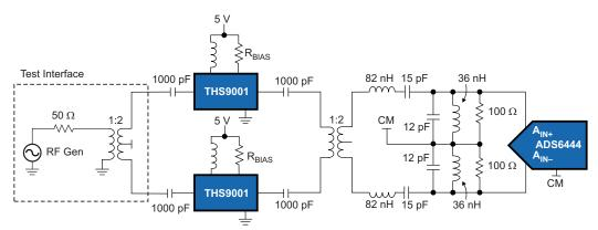
Figure 20. High-Speed A/D Driver Amplifier (Based on the THS9001)
