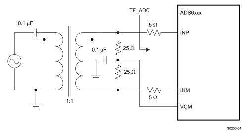
Figure 2. Example of a Passive Single Transformer Drive Circuit for an Unbuffered Analog Input
