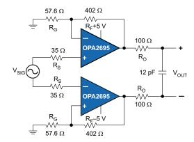
Figure 13. Differential Noninverting Amplifier
