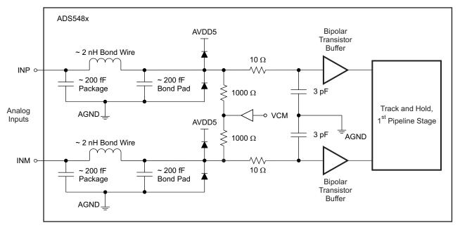
Figure 5. Example of an Equivalent Model of a Buffered Analog Input
