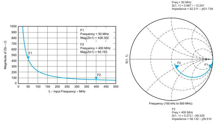
Figure 4. Differential Input Impedance vs Frequency for an Unbuffered Sample-and-Hold Input
