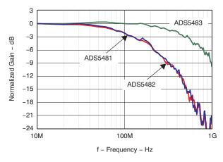
Figure 7. Analog Input Response of the ADS5481/2/3 Family
