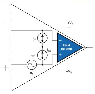
Figure 10. Input-Referred Op Amp Noise Model
