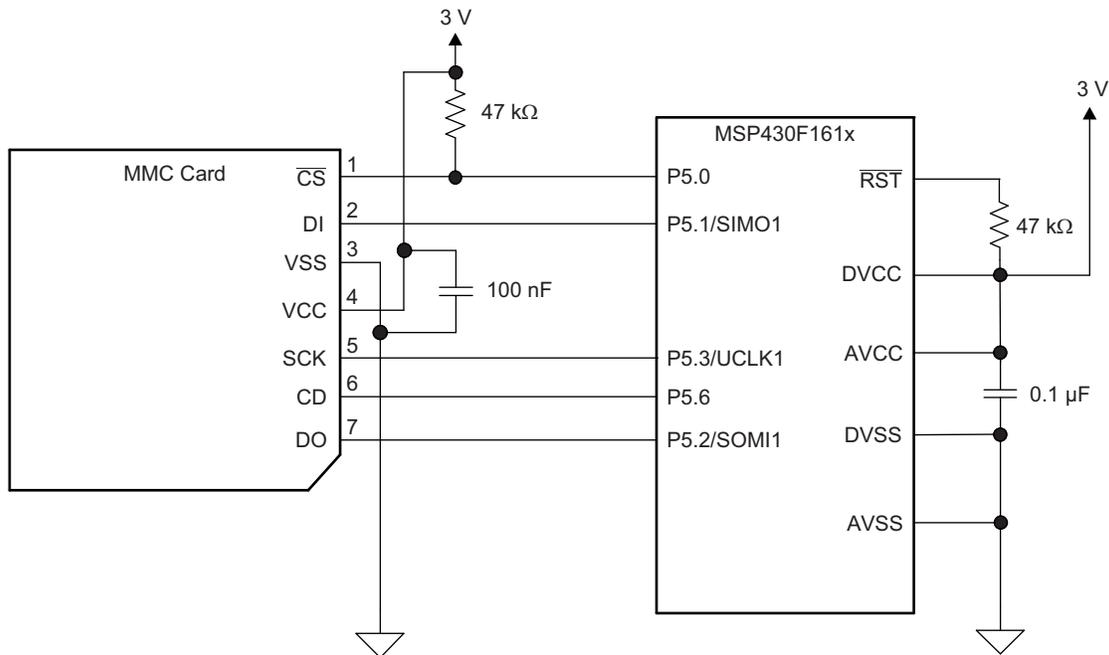
**Figure 1. Connection Between MSP430 MCU and MMC Card**
