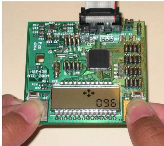
**Figure 8. Picture of EKG Board in Action**
