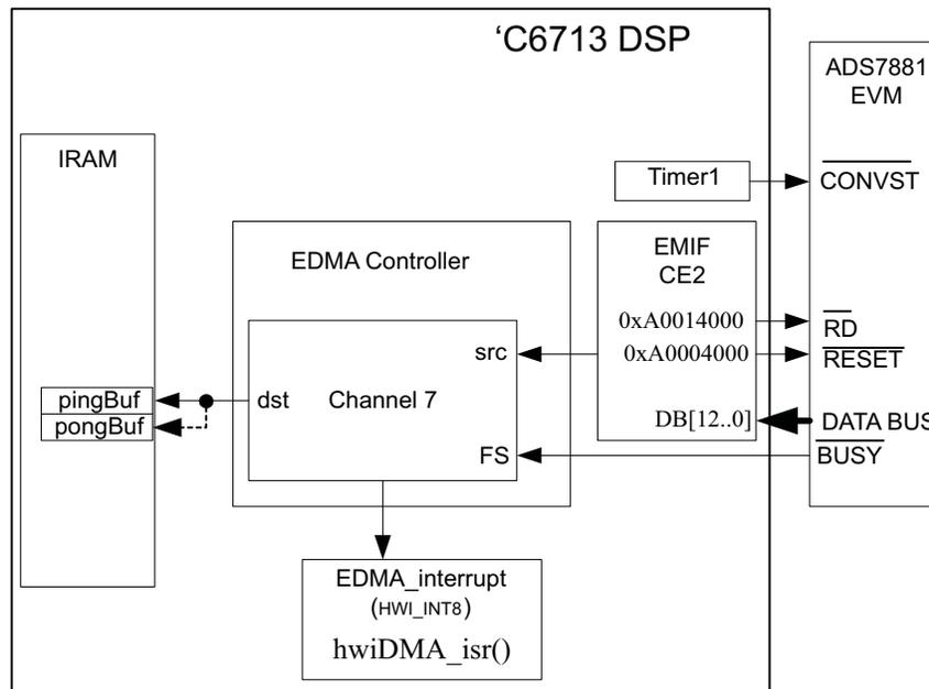
Figure 2. Data Transfer Block Diagram Using EDMA
