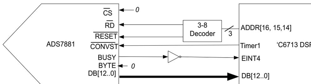
**Figure 1. Hardware Connection**
