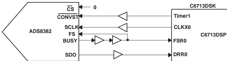
Figure 1. Hardware Connection
