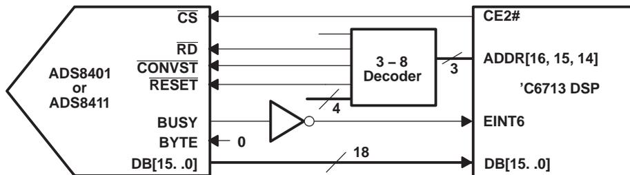
**Figure 1. Hardware Connection**
