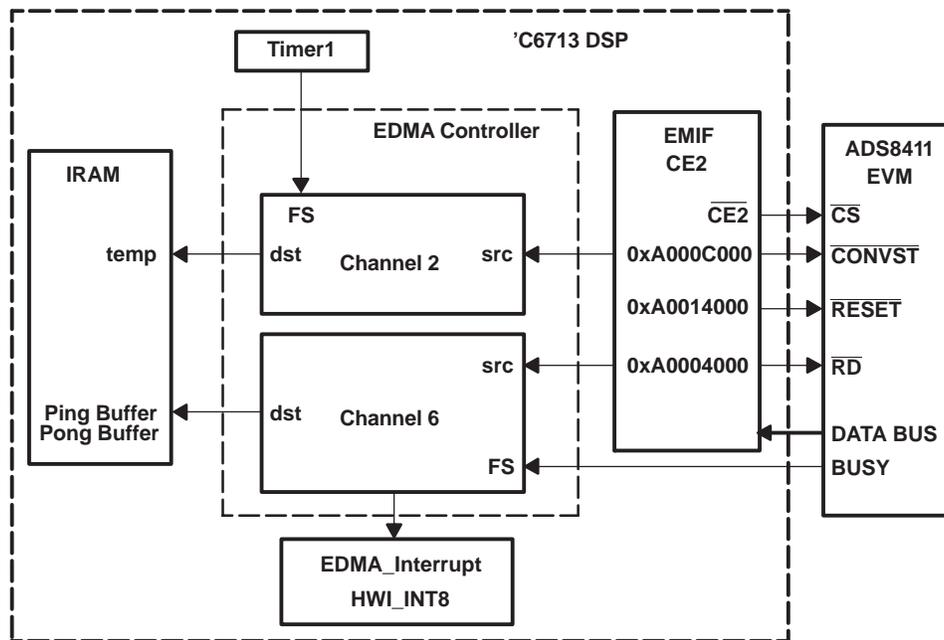
**Figure 2. Data Transfer Block Diagram Using EDMA**
