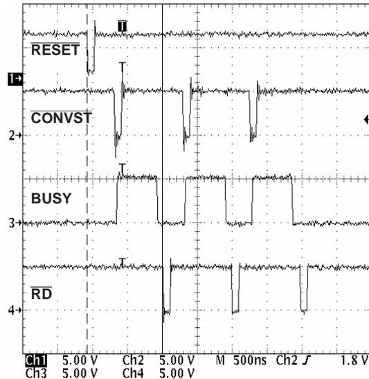
**Figure 4. Scope Screenshot Showing Power-on Initialization Cycles**
