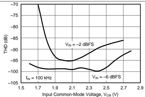
**Figure 13. Total Harmonic Distortion vs Input Common-mode Voltage**
