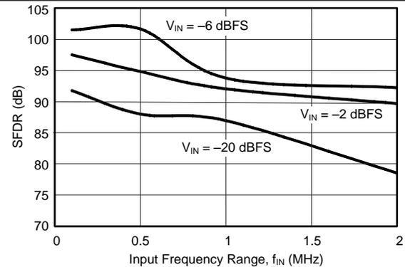
**Figure 11. Spurious Free Dynamic Range vs Input Frequency**
