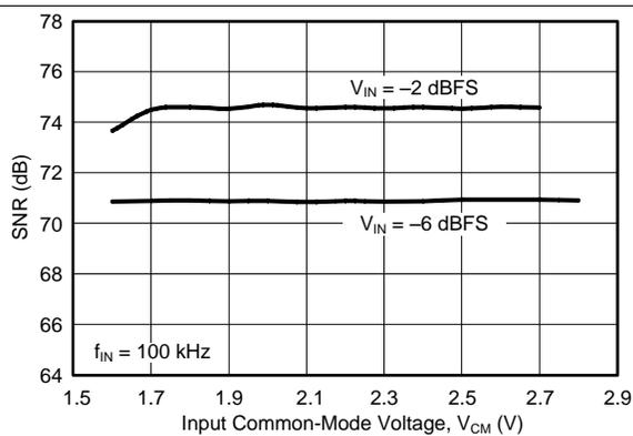
**Figure 12. Signal-to-Noise Ratio vs Input Common-Mode Voltage**
