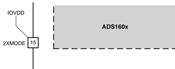
**Figure 1. Pin Configuration for Doubling Output Data Rate**
