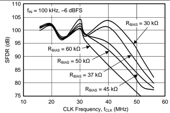
**Figure 17. Spurious-Free Dynamic Range vs CLK Frequency**
