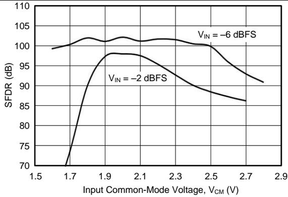
**Figure 14. Spurious-Free Dynamic Range vs Input Common-Mode Voltage**
