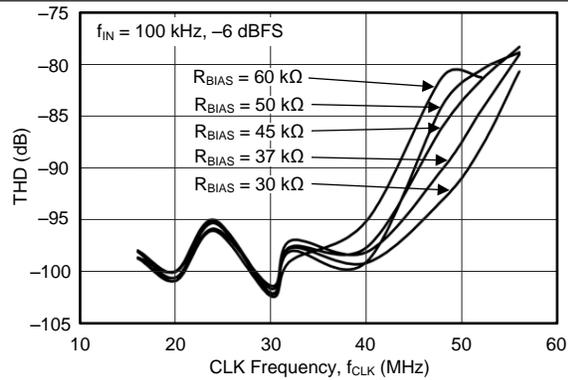
**Figure 16. Total Harmonic Distortion vs CLK Frequency**
