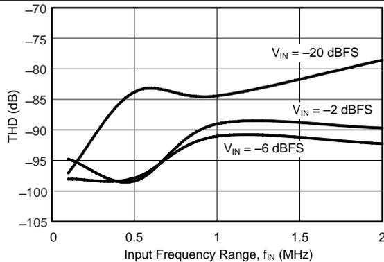
**Figure 10. Total Harmonic Distortion vs Input Frequency**
