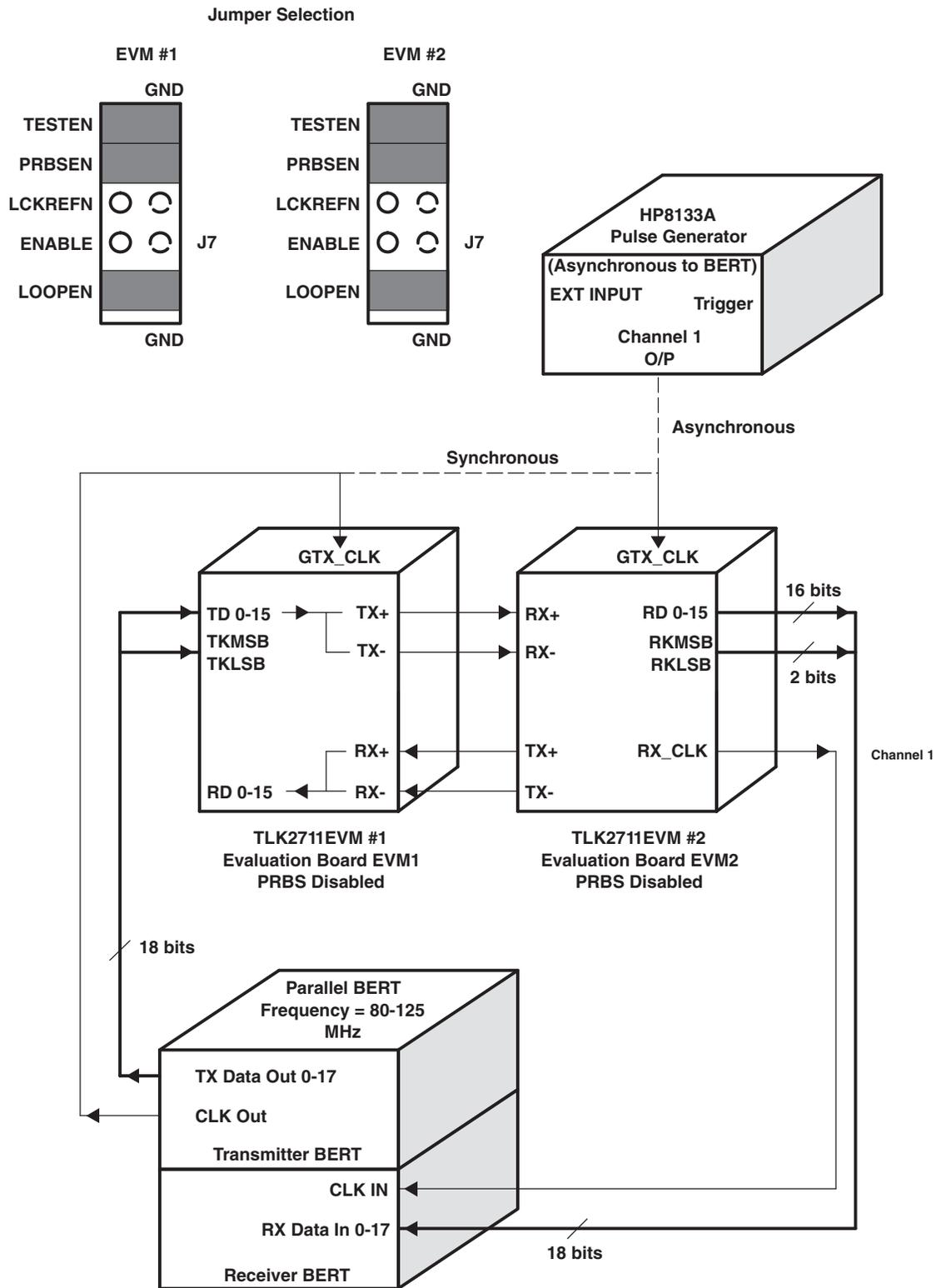
**Figure 2-4. TLK2711 Serial PRBS BERT Test Configuration**
