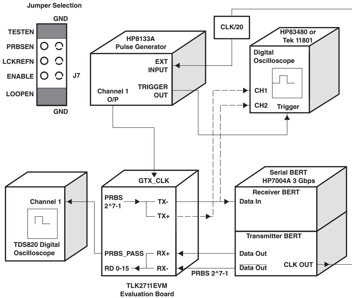
Figure 2-3. TLK2711 Serial PRBS BERT Test Configuration
