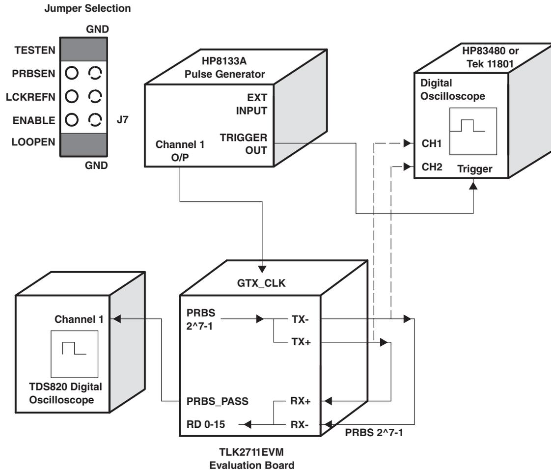
**Figure 2-2. TLK2711 Serial Loop-Back Test Configuration**
