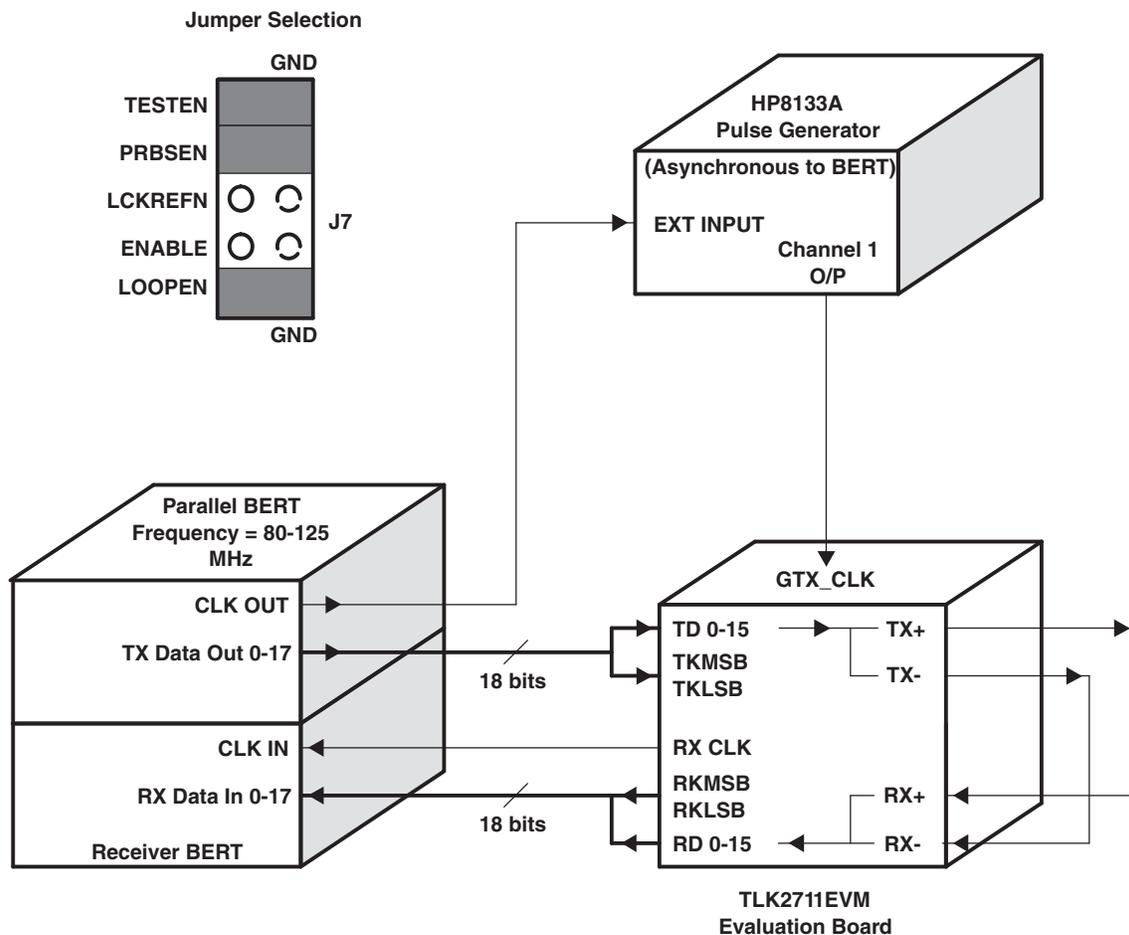
Figure 2-1. TLK2711 Serial Loop-Back Test Configuration
