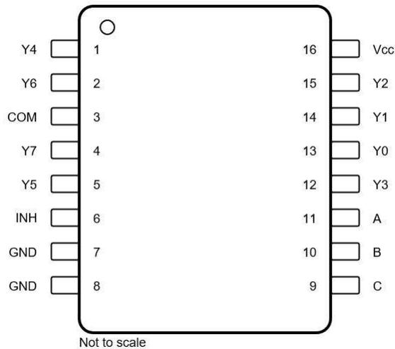
**Figure 4-1. Pin Diagram TSSOP and SOIC Packages**
