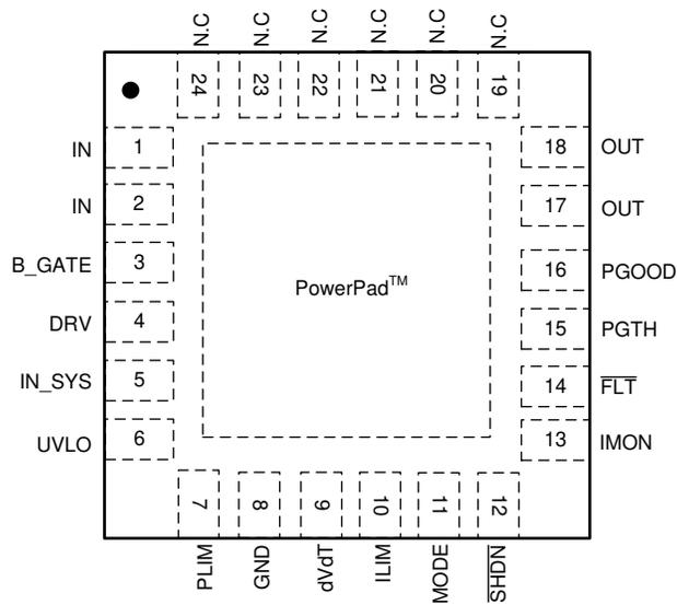
**Figure 4-2. TPS26632, TPS26633, TPS26635 Pin Diagram (VQFN) Package**
