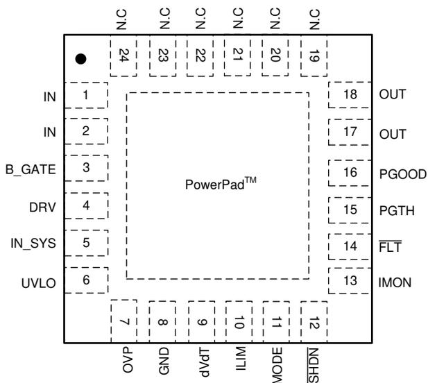
**Figure 4-1. TPS26630, TPS26631 Pin Diagram (VQFN) Package**
