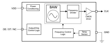
Figure 1-1. Functional Block Diagram
